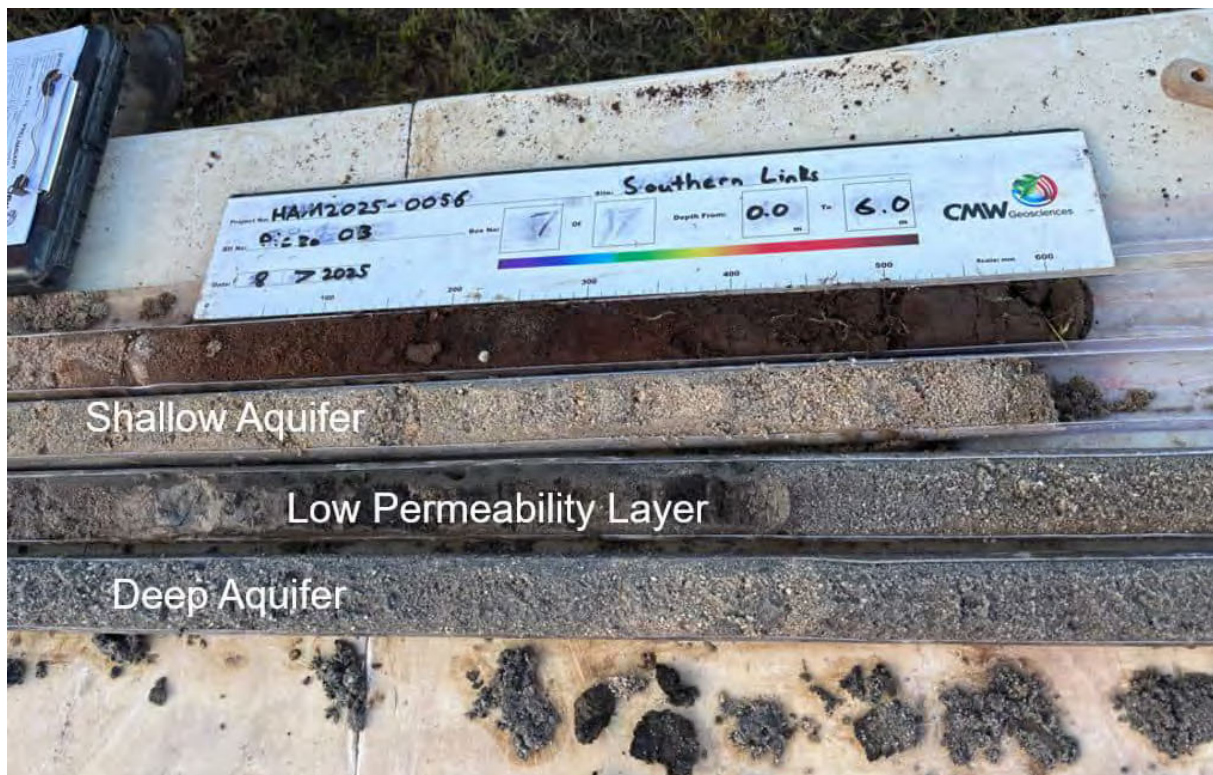
Figure 9: Field Identification of Lithological Units Present at Bore P3
