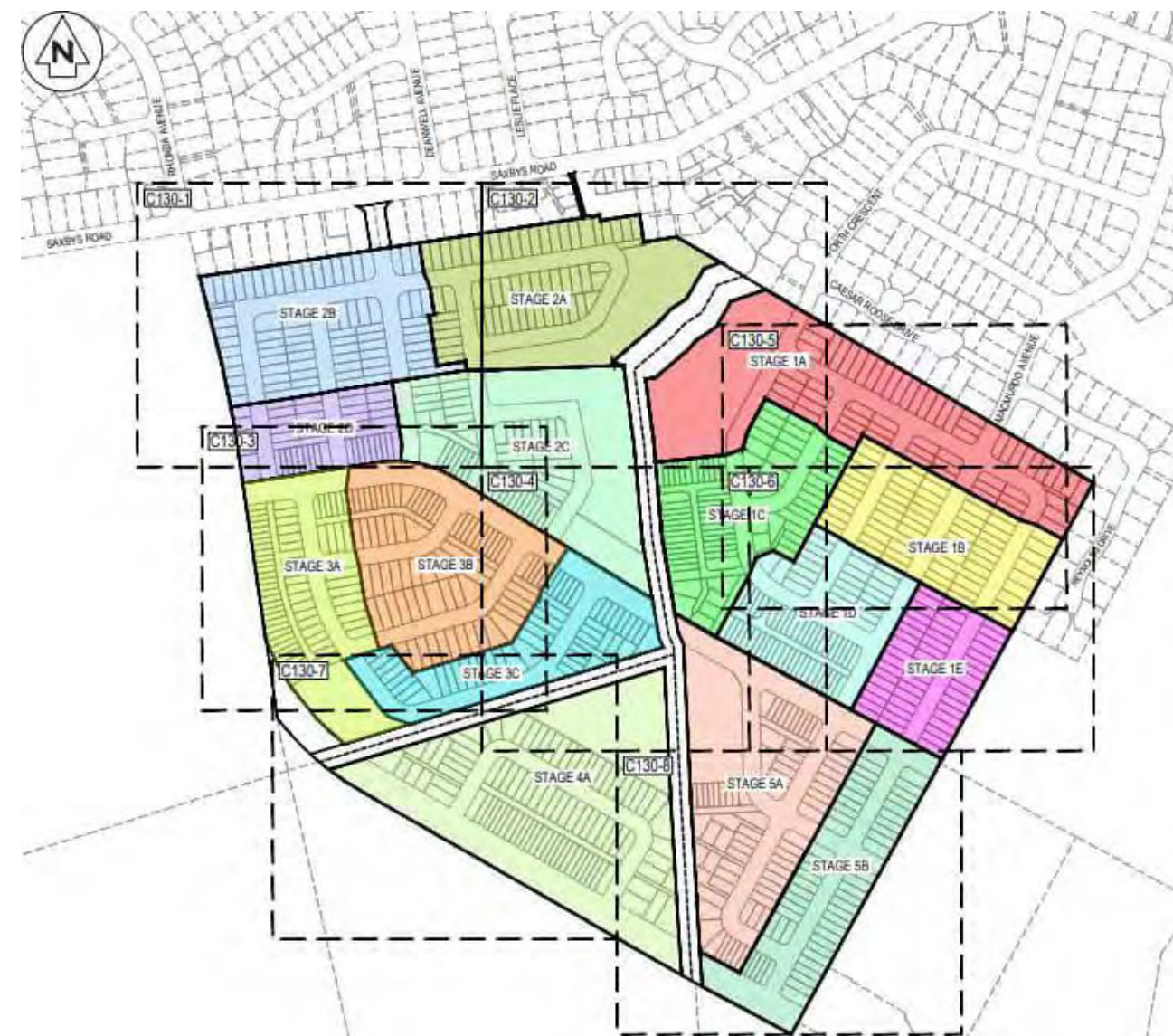
Figure 2: Proposed Staging Plan prepared by Maven (Ref: 298001-R1 SL1, Drawing No: R1-C130 Rev A, dated June 2026)
