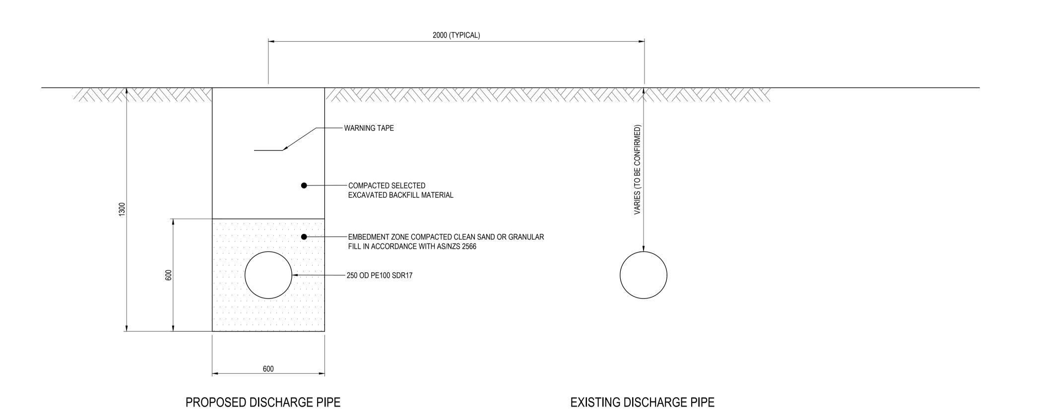
TYPICAL DISCHARGE PIPE SECTION
