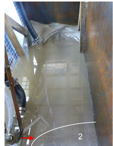
Figure 8: Low grade dense including slewing, jets v_z=0.6 cm/sec resulting in steps of 2,5 cm (Test 3.21)
