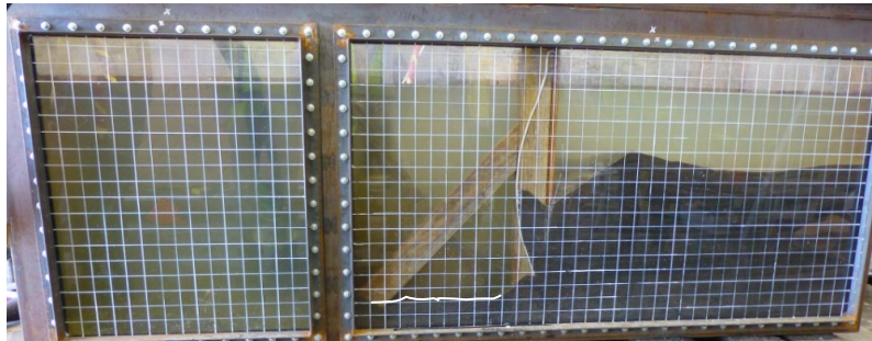
Figure 8: Low grade dense including slewing, jets v_z=0.6 cm/sec resulting in steps of 2,5 cm (Test 3.21)
