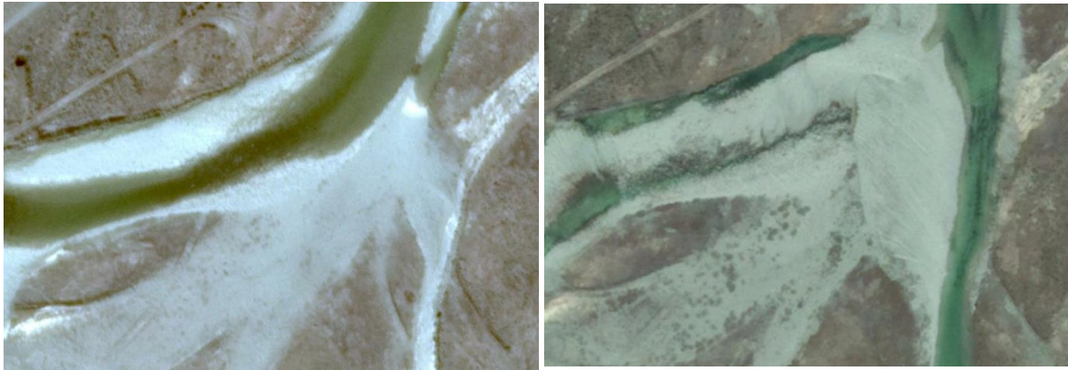
Figure 1: Google Earth aerial showing river works on the Takapō River riverbed, (left) 2012 riverbed, (right) 2016 riverbed with main braid diversion.
