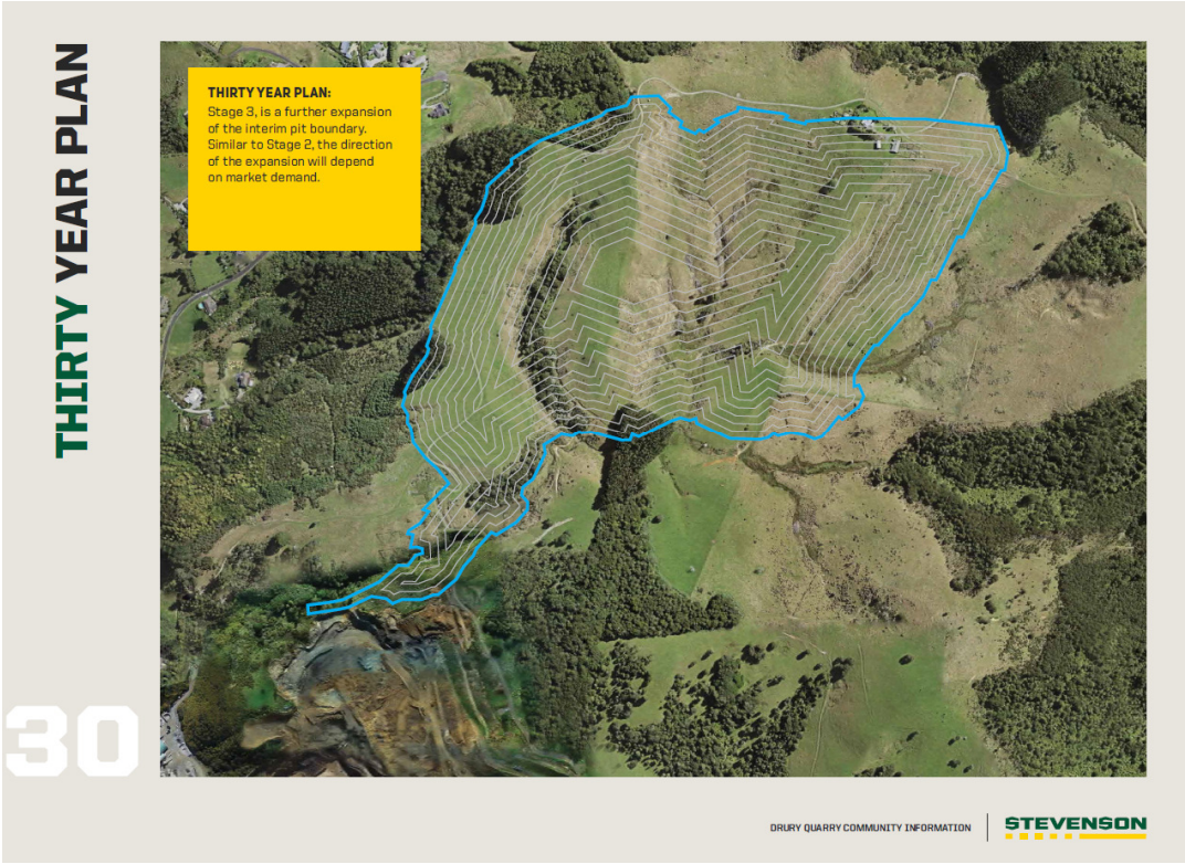
Figure 3: Stage 3 - Interim pit boundary
