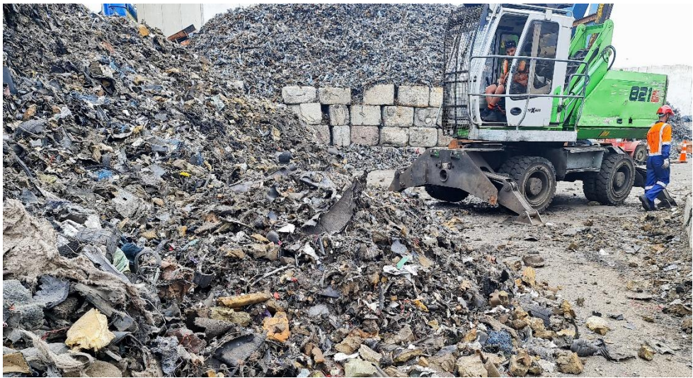
Figure B: Recovered floc material, post shredding, stockpiled at National Green Steel’s processing and recovery plant in Manukau, Auckland.
