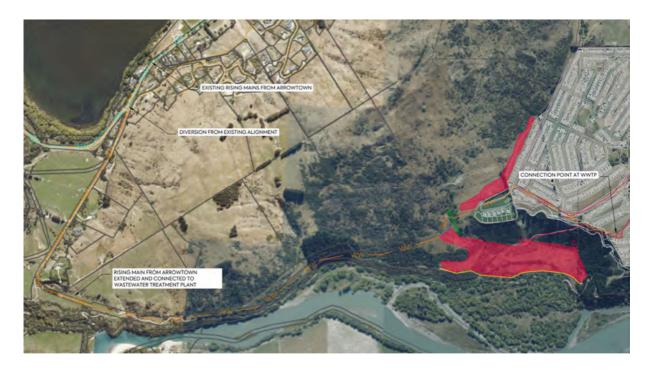
Figure 5: Potential route for a wastewater pipe from the existing network, to alleviate flows in existing system.
