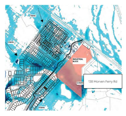
Figure 2 - Pre-Development Flows - 1% AEP including 3.8-degree climate change.
