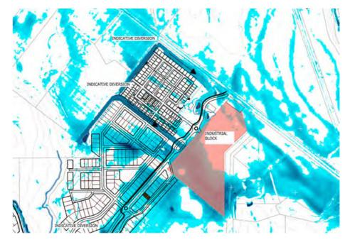
Figure 4 - Option for flood Mitigation to pass upstream flows through the site.
