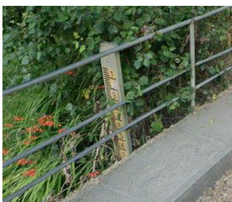
Figure 1: Example of a permanent visual water level monitor
