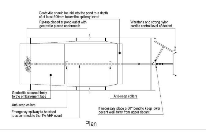
FIGURE 72 GD05 - SEDIMENT RETENTION POND (UP TO 3.0ha CATCHMENT PER POND)
