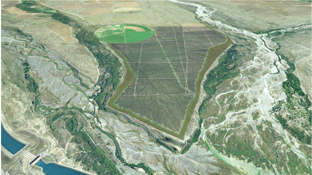
Overview of 3D model showing digital terrain model with solar panel layout and landscaping.
