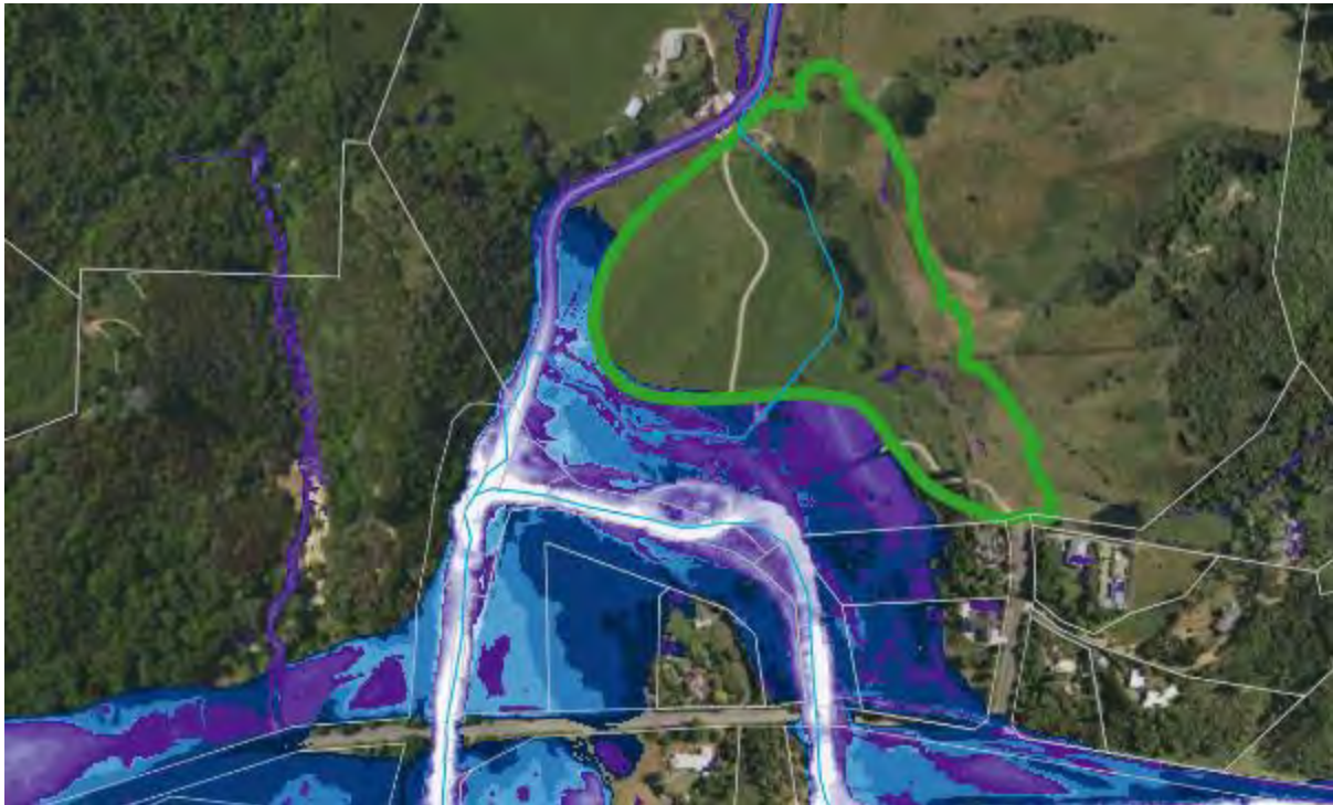
Figure 5.8: Modelled post-development scenario, including restored and enhanced Kākā Stream, proposed flood plain earthworks as per green polygon, and unattenuated post-development flows from developed catchment (2130 RCP8.5M 1% AEP 6hr event in blue, 10% AEP event in purple).
