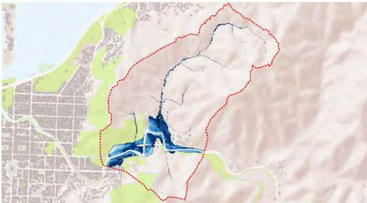
Figure 2.5: Flood depth mapping within the Kākā Stream Catchment in blue – 2130 RCP8.5 1% AEP 6-hour event. The red dashed line is the model boundary.
