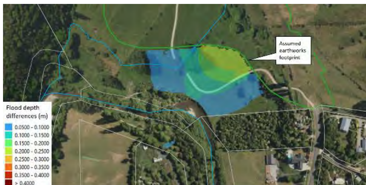
Figure 5.7: Extent of local increase in flood depths as a result of proposed filling (2130 RCP8.5M 1% AEP 12hr event).
