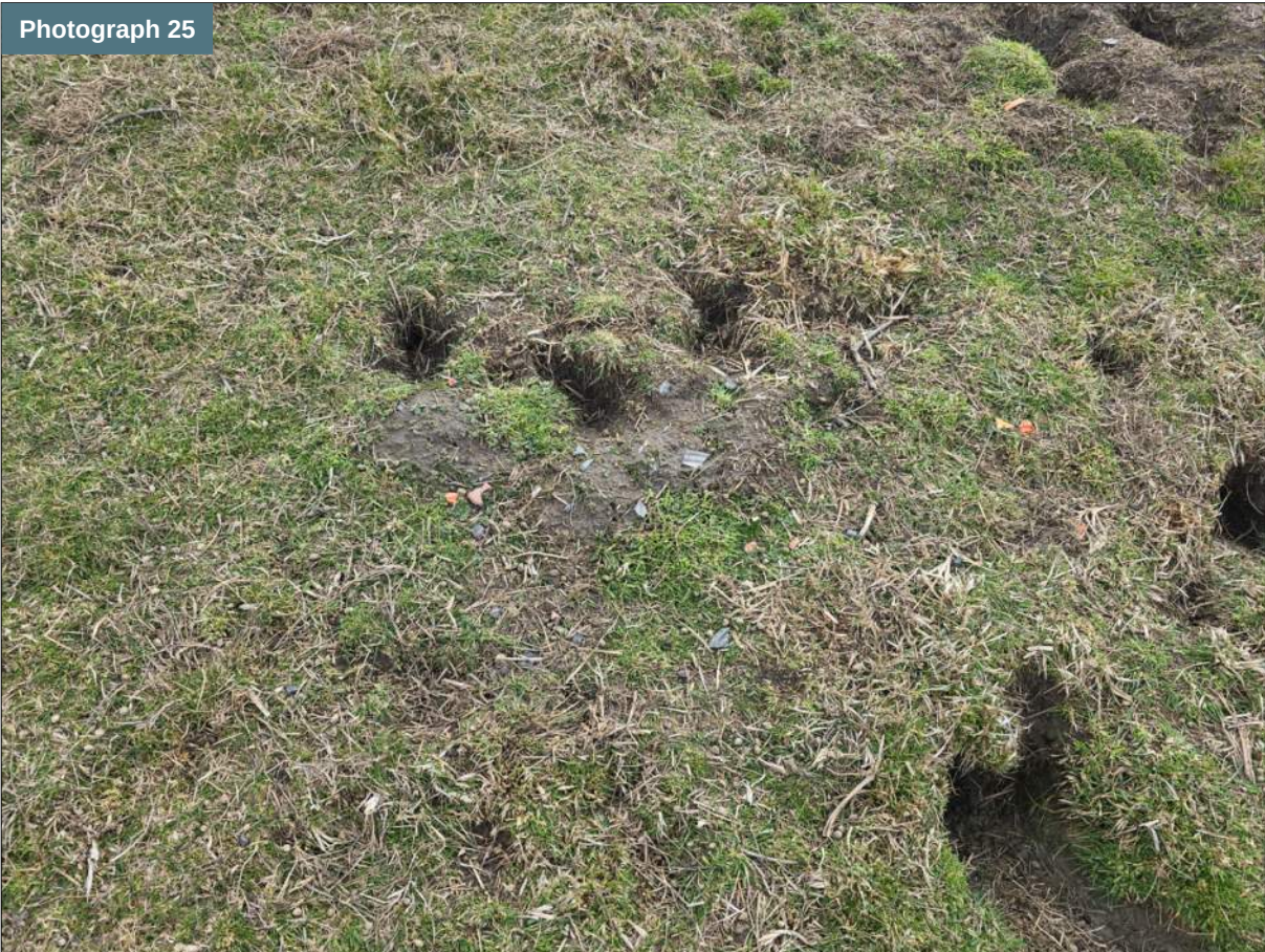
Soil surface on the hillside facing the firing range with visible clay fragments and lead pellets. (Area 2)
