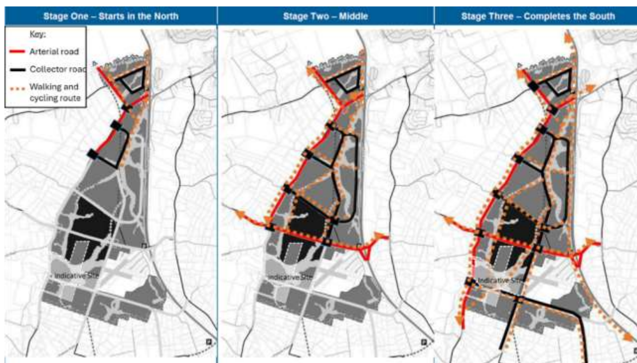
Figure 14: Indicative Structure Plan transport sequencing (sourced from Structure Plan ITA by Te Tupu Ngātahi, March 2019). Site indicated in white
