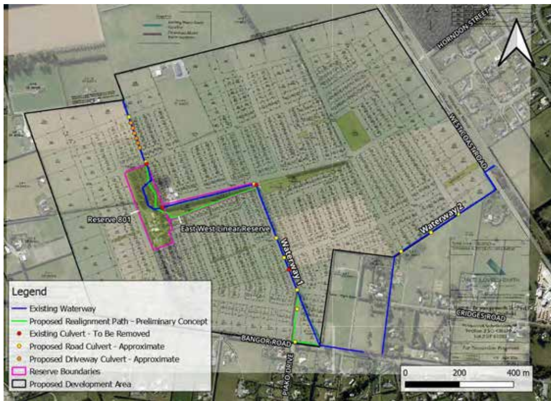
Figure 2 – Proposed realignment and culvert works.
