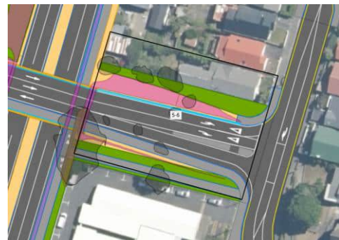
Figure 69 Moxham Avenue buildings requiring demolition (Feature 5-6)
