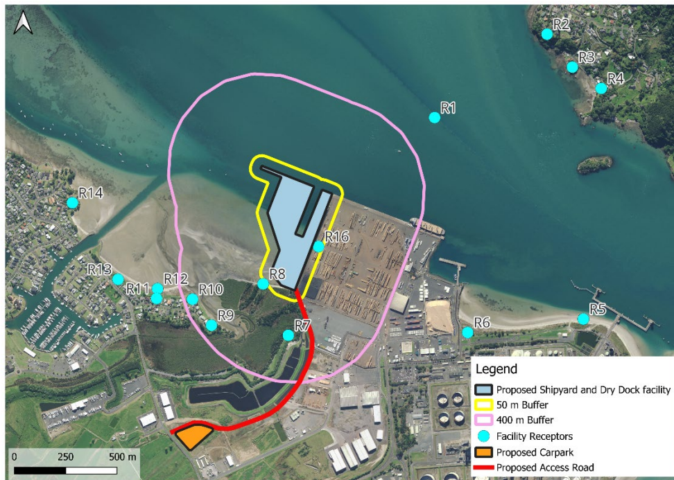
Figure 14: General Mitigated and Unmitigated Dust Transportation Areas for Shipyard and Dry Dock Facility
