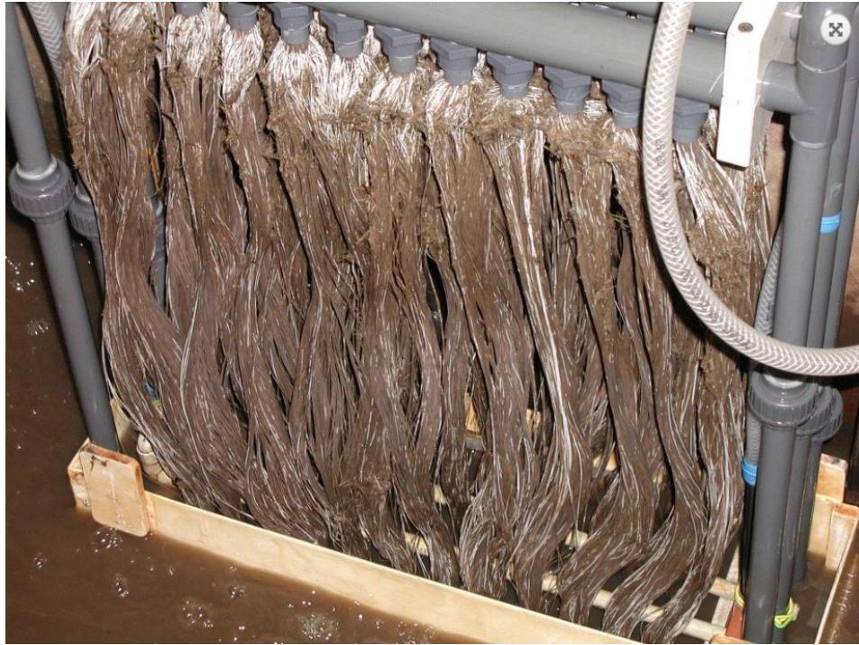
Figure 29 - An example of fouling on hollow fibre membranes (Bates, 2018)
