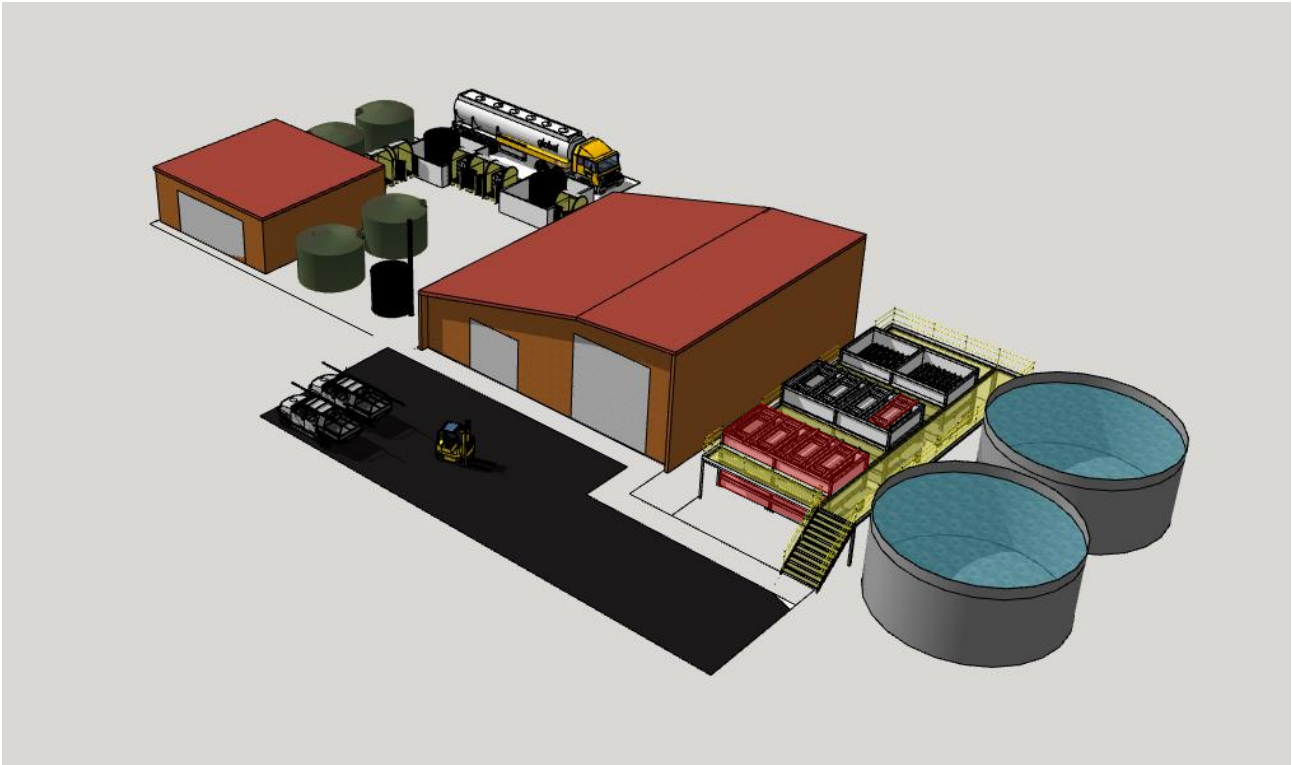
Figure 14 - Pre-Anoxic Tank and MABR Modules that can be installed at a later date (highlighted in red)
