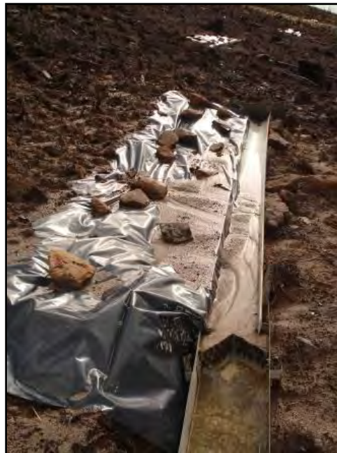
Figure 10. Erosion control gutter used to measure sediment loss from trial plots. Further details of the design, methodology, and results are available (Shadbolt and Weber, 2007).
