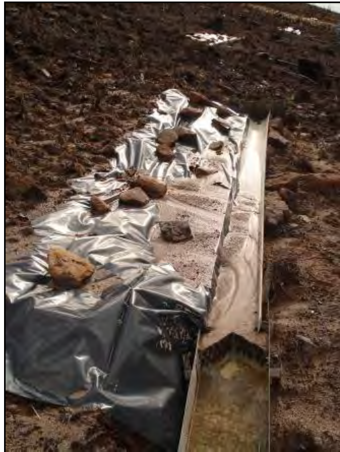
Figure 1. Catch trough showing upslope polythene sheeting and mesh filter/splitter at the outflow.
