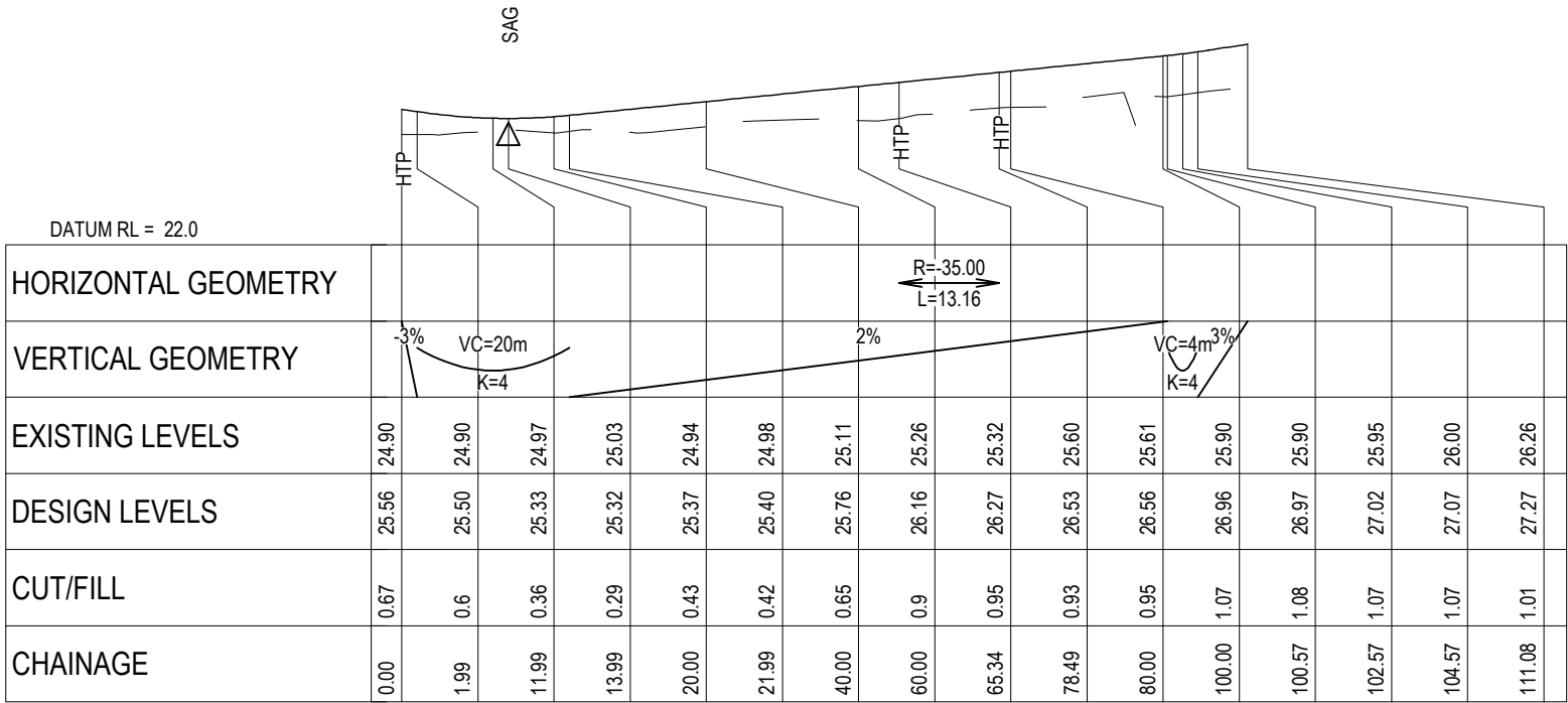
ROAD 18 LONGITUDINAL SECTION SCALE HORI 1:1000 VERT 1:200
