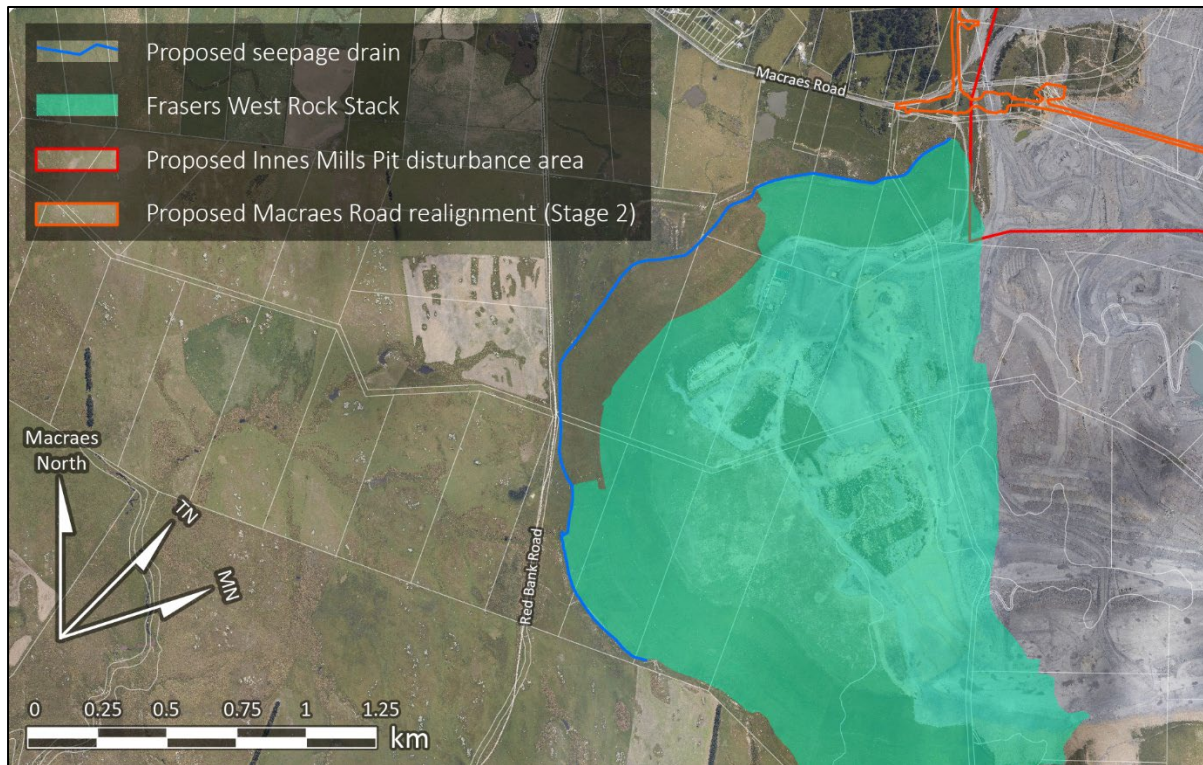
Figure 15. Seepage drain around the around Frasers West Waste Rock Stack (2025 OGNZL aerial photography).
