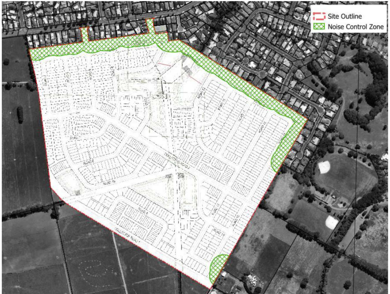
Figure 1 Noise Control Zone – all construction work within this area must be managed to comply with the noise limits.
