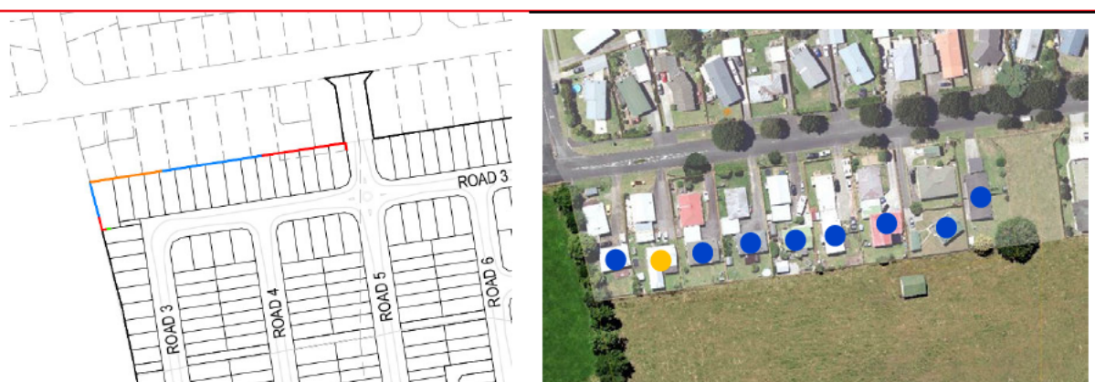
Figure 5 Retaining wall construction: receivers predicted to experience noise levels of up to 75 dB L_{Aeq} (blue circle) and 80 dB L_{Aeq} (orange circle)
