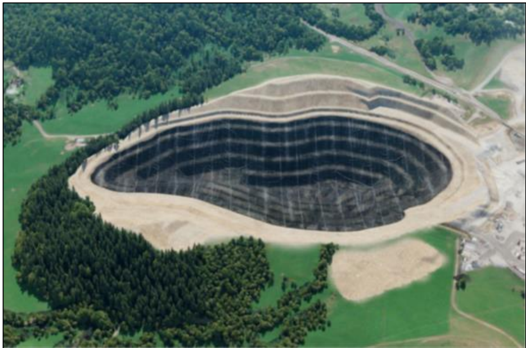
Figure 2-42: Isometric View of the GOP TSF Prior to Tailings Input
