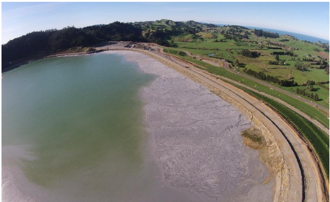
FIGURE 25: STORAGE 1A TAILINGS SURFACE WITH PONDED WATER MANAGED BY OGNZL THROUGH THE WATER TREATMENT PLANT
