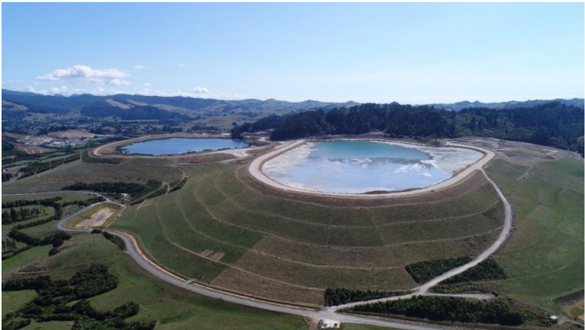
FIGURE 3: AERIAL PHOTO OF STORAGE 2 (LEFT) AND STORAGE 1A (RIGHT) WHICH STORE THE TAILINGS AT THE WAIHI OPERATION
