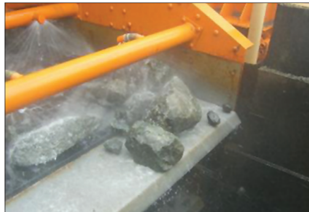
Figure 21—Vibrating sizing screen with example oversize material
