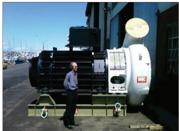
Figure 19—IHC underwater pump and eMotor for crawler application
