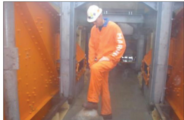
Figure 18—Boulder hydrohoisted by airlift (approximately 450 mm max dimension)
