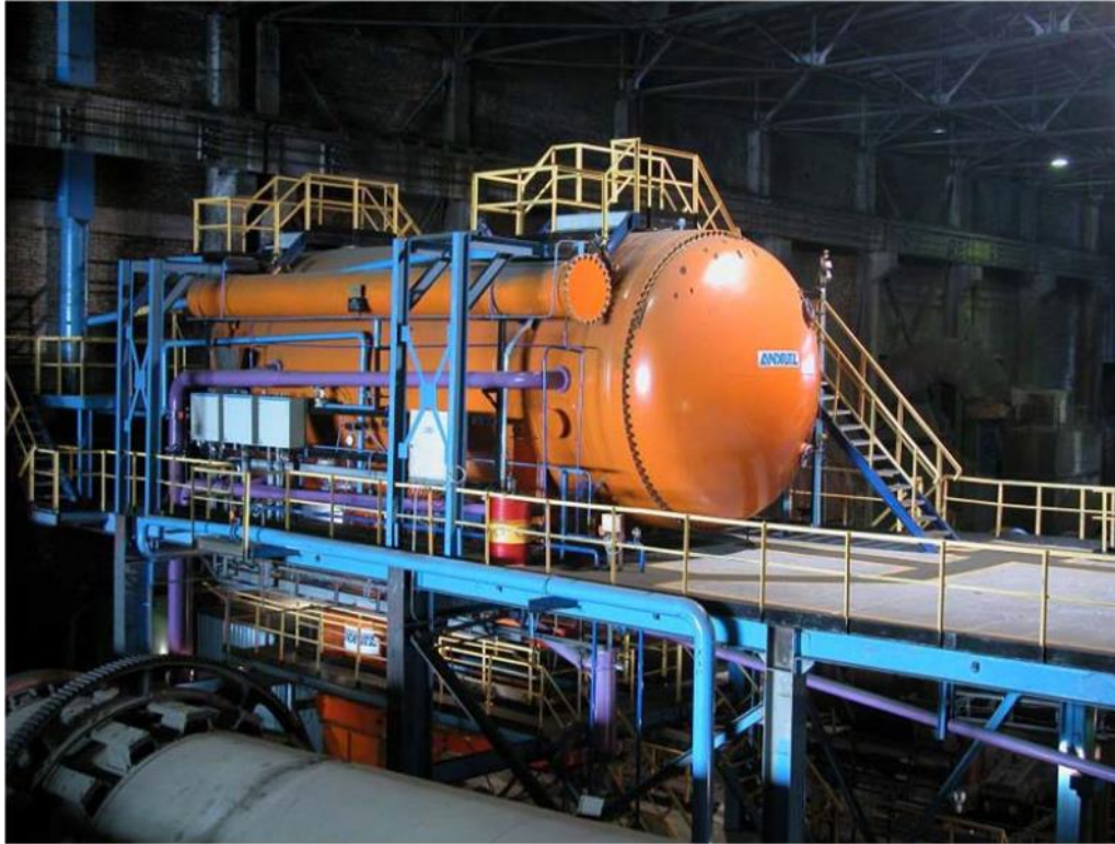
Figure 2.9: Example of the Hyperbaric Pressure Filter
