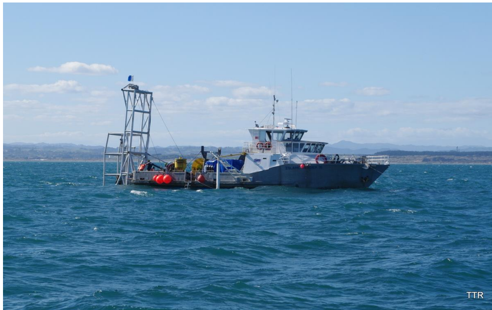
Figure 2.5: The Island Leader II. Used by TTR for offshore drilling in the South Taranaki Bight.
