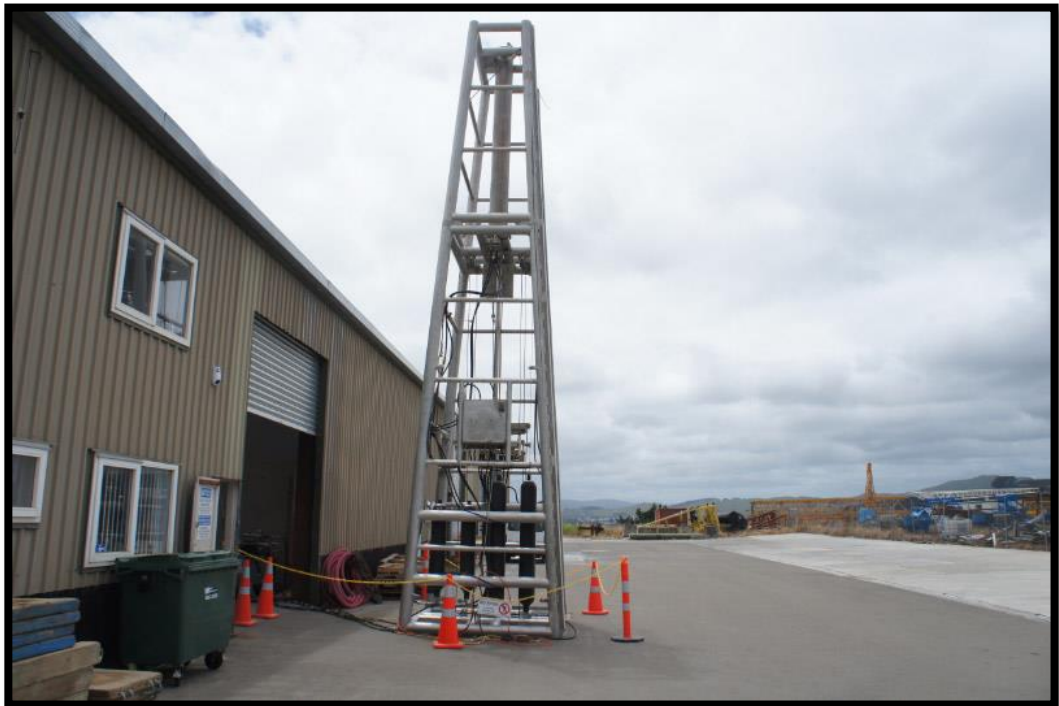
Figure 2.4: The drill rig that will be used in grade control drilling
