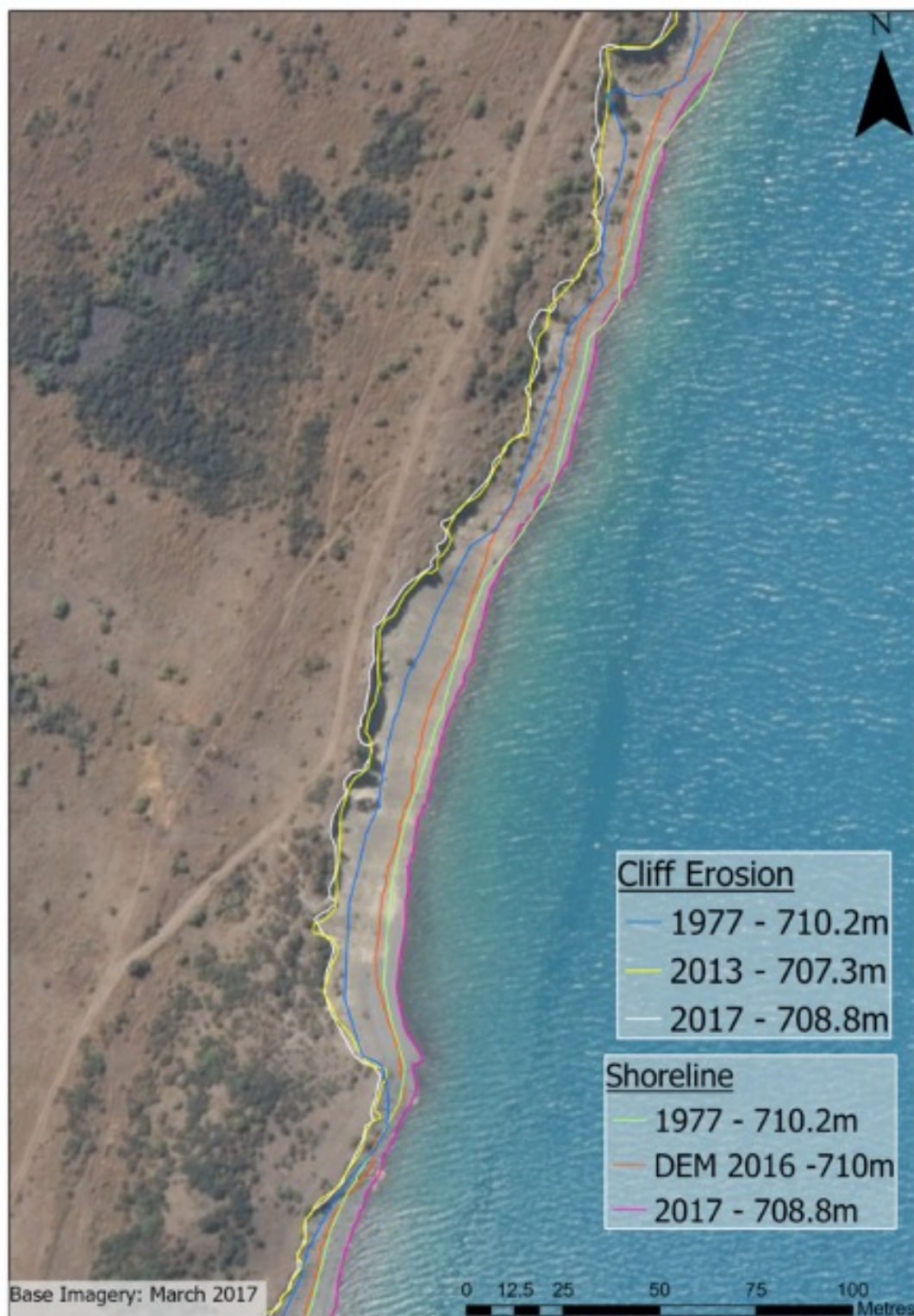
Figure 3.5 Changes in scarp top and shoreline position adjacent to the northern Mt John walkway
