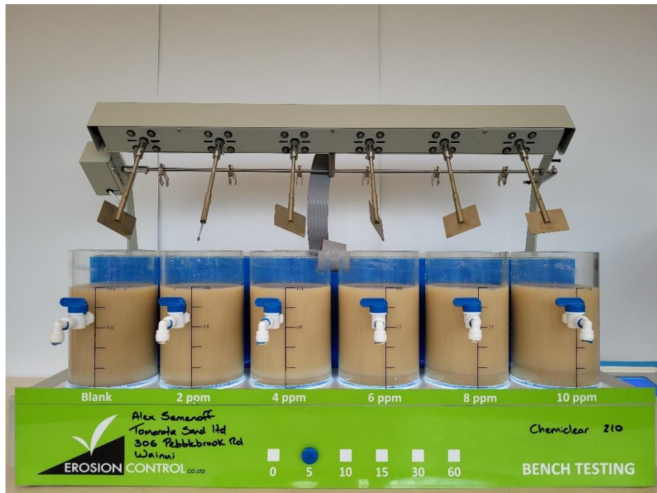
CATCHMENT SAMPLE: Test Results of Chemiclear 210 after 5 minutes settling
