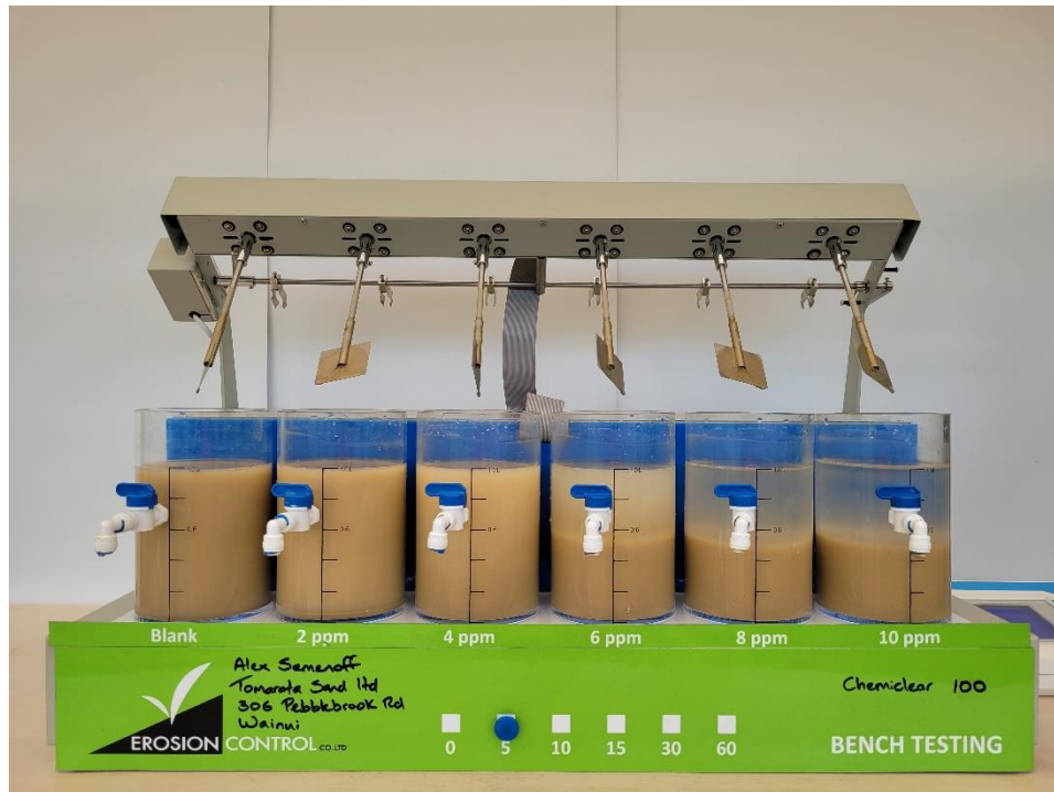
CATCHMENT SAMPLE: Test Results of Chemiclear 100 after 5 minutes settling
