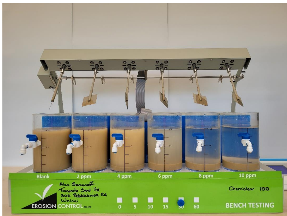
CATCHMENT SAMPLE: Test Results of Chemiclear 100 after 30 minutes settling
