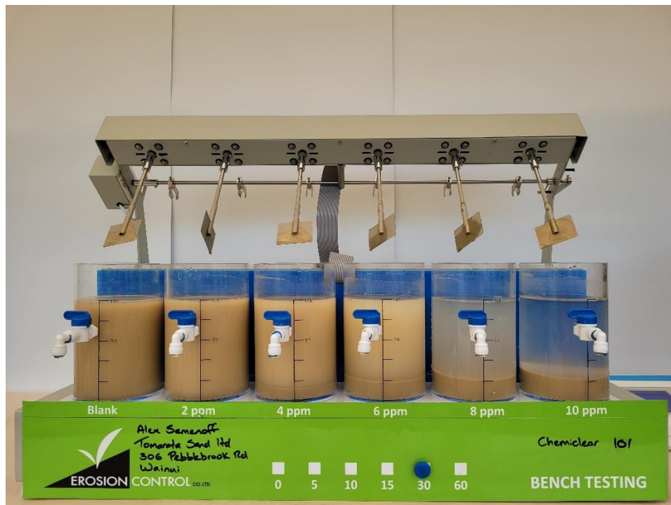
CATCHMENT SAMPLE: Test Results of Chemiclear 101 after 30 minutes settling
