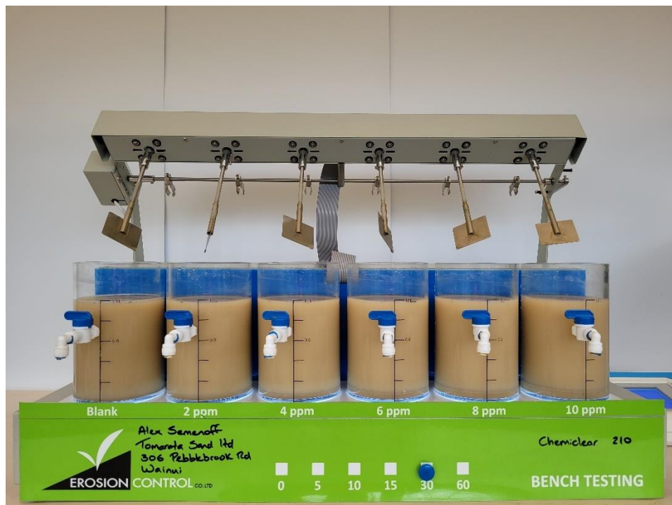
CATCHMENT SAMPLE: Test Results of Chemiclear 210 after 30 minutes settling
