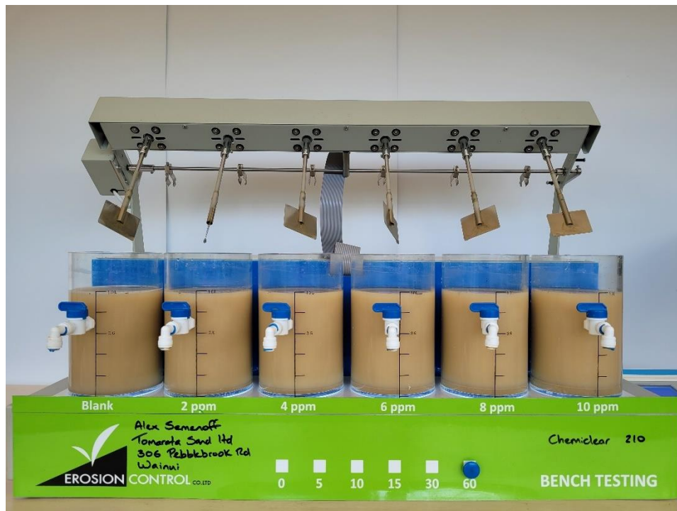
CATCHMENT SAMPLE: Test Results of Chemiclear 210 after 60 minutes settling
