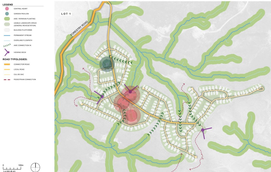
Figure 24: Landscape Strategy diagram illustrating the way in which the site of the retirement village is tied into the landscape with revegetated riparian corridor fingers / awe (tassels) extending up into the village, creating neighbourhoods.
