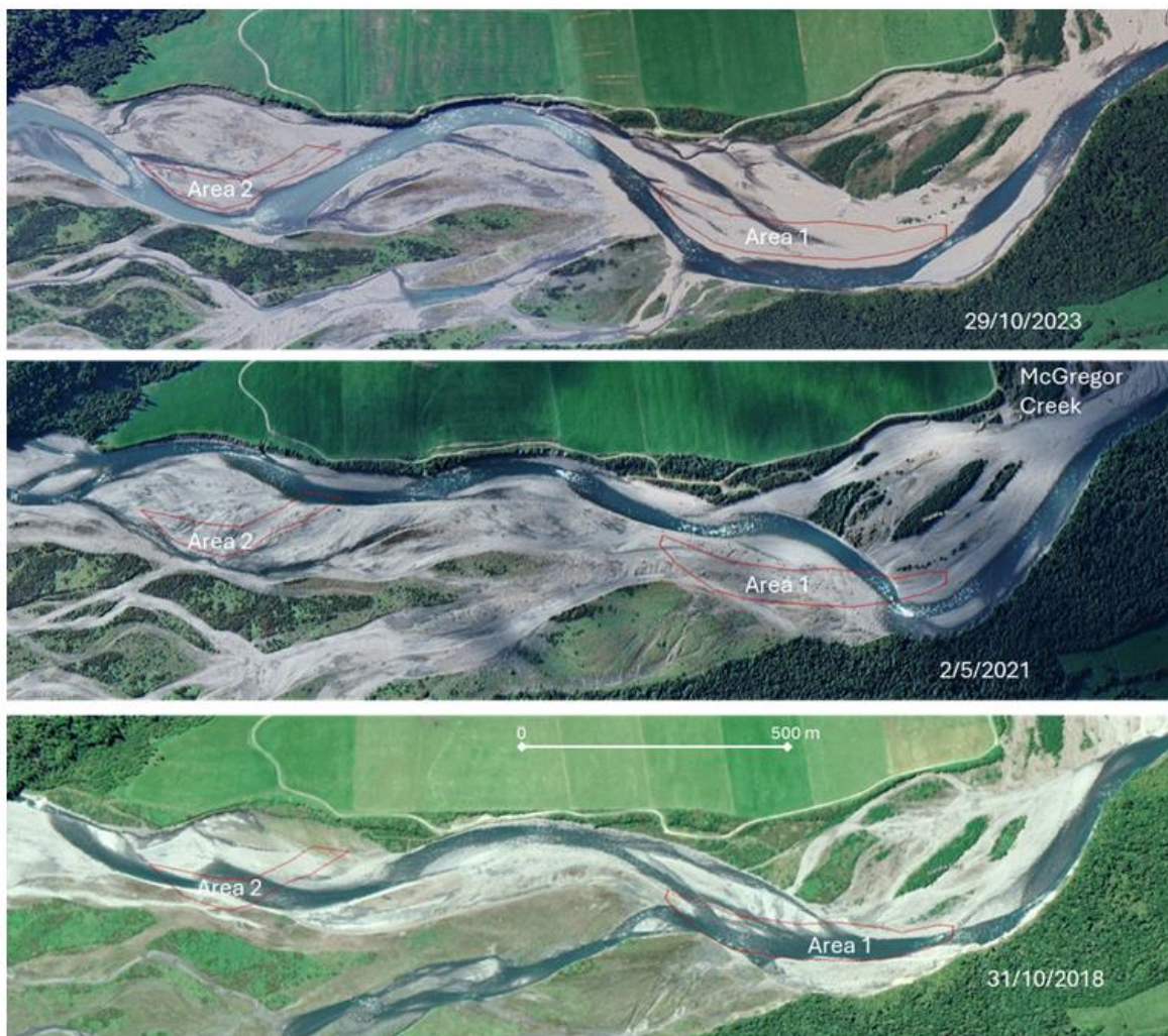
Figure E-9: Gravel borrow-area 1 and 2 locations (red outlines) on Waitaha active braidplain downstream from Macgregor Creek as originally proposed. While dry and accessible from northern bank on 29/10/2023, on 2/5/2021 these areas were on the south side of the Waitaha main channel and on 31/10/2018 they were in the main channel. Current proposal recognises that borrow-areas will need to be located according to braid and bar locations at the time of extraction. Borrow-areas shown taken from Westpower Plans Waitaha River proposed new power scheme gravel take areas for the road construction etc, Waitaha Area 1 (Wed Feb 5 11:04:11 2025) and Waitaha River proposed new power scheme gravel take areas for the road construction etc, Waitaha Area 2 (Wed Feb 5 11:04:44 2025).
