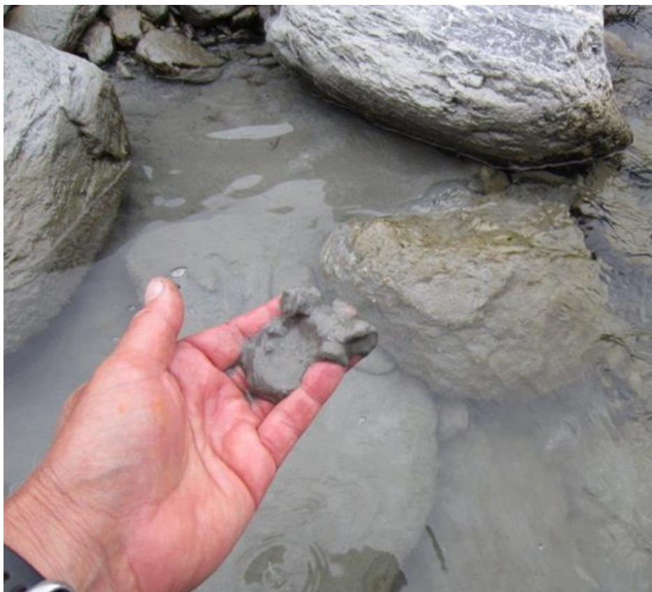
Figure 2-3: Silty sludge draped over/among channel margin cobbles at Kiwi Flat during baseflow of 8–10 m³/s that had persisted for at least 23 days in February 2013.
