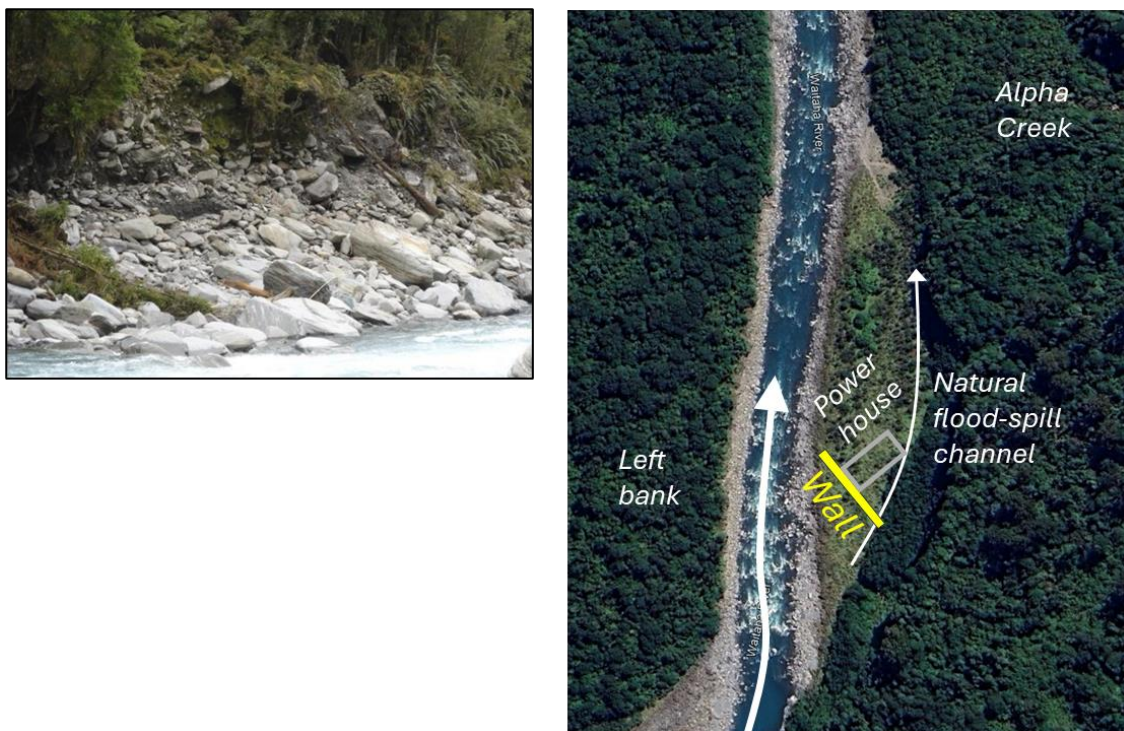
Figure 2-5: Right – schematic showing natural flood-spill channel and floodwall on the terrace where the Power Station will be located. Left – the Waitaha left bank, with a boulder lag on its lower slope.
