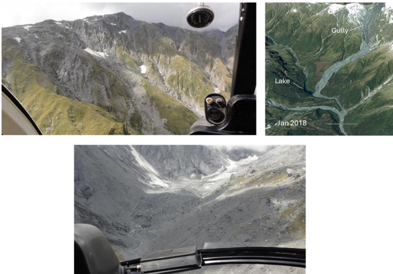
Figure 2-1: Typical sediment sources in the Waitaha Catchment. Top-left: Debris mantled slopes and gullies in Waitaha headwaters. Top-right: Gully complex and debris chute in County Stream reactivated between September 2016 and January 2018, damming a lake that stalled sediment delivery from Upper County Stream (image: Google Earth). Bottom: View up-valley of the sediment-draped County Glacier issuing turbid meltwater, upper Waitaha.
