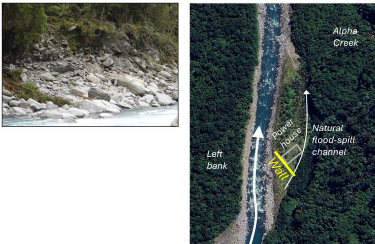
Figure D-10: Waitaha bank at Power Station site. Left: the left bank with a boulder lag on its lower slope. Right: schematic showing natural flood-spill channel and floodwall on the terrace where the Power Station is proposed to be located.
