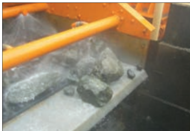
Figure 21—Vibrating sizing screen with example oversize material
