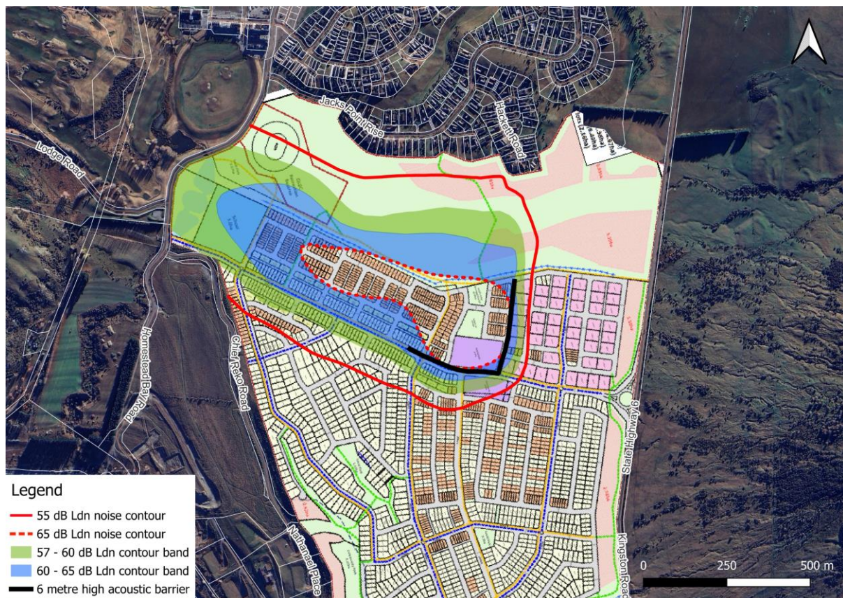
Figure 5.1 – Noise level with 6-metre-high acoustic barrier
