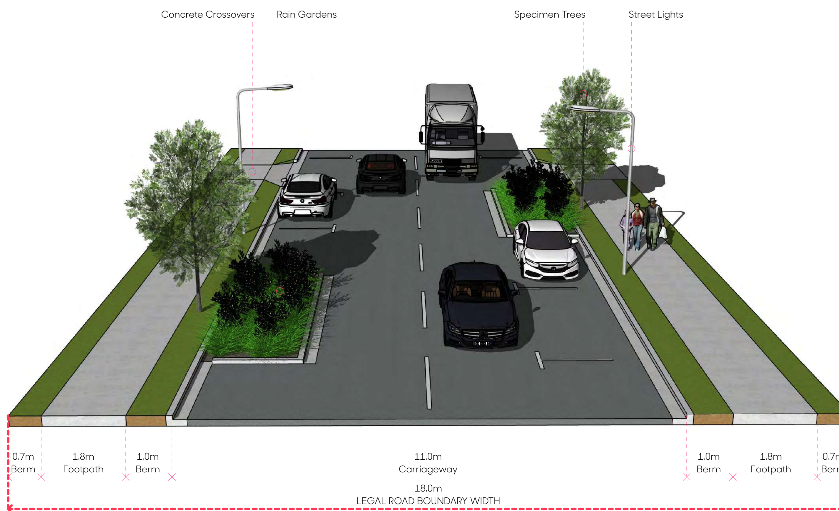
TYPICAL SECTION : 18M ROAD 1:50@A1 / 1:100@A3
