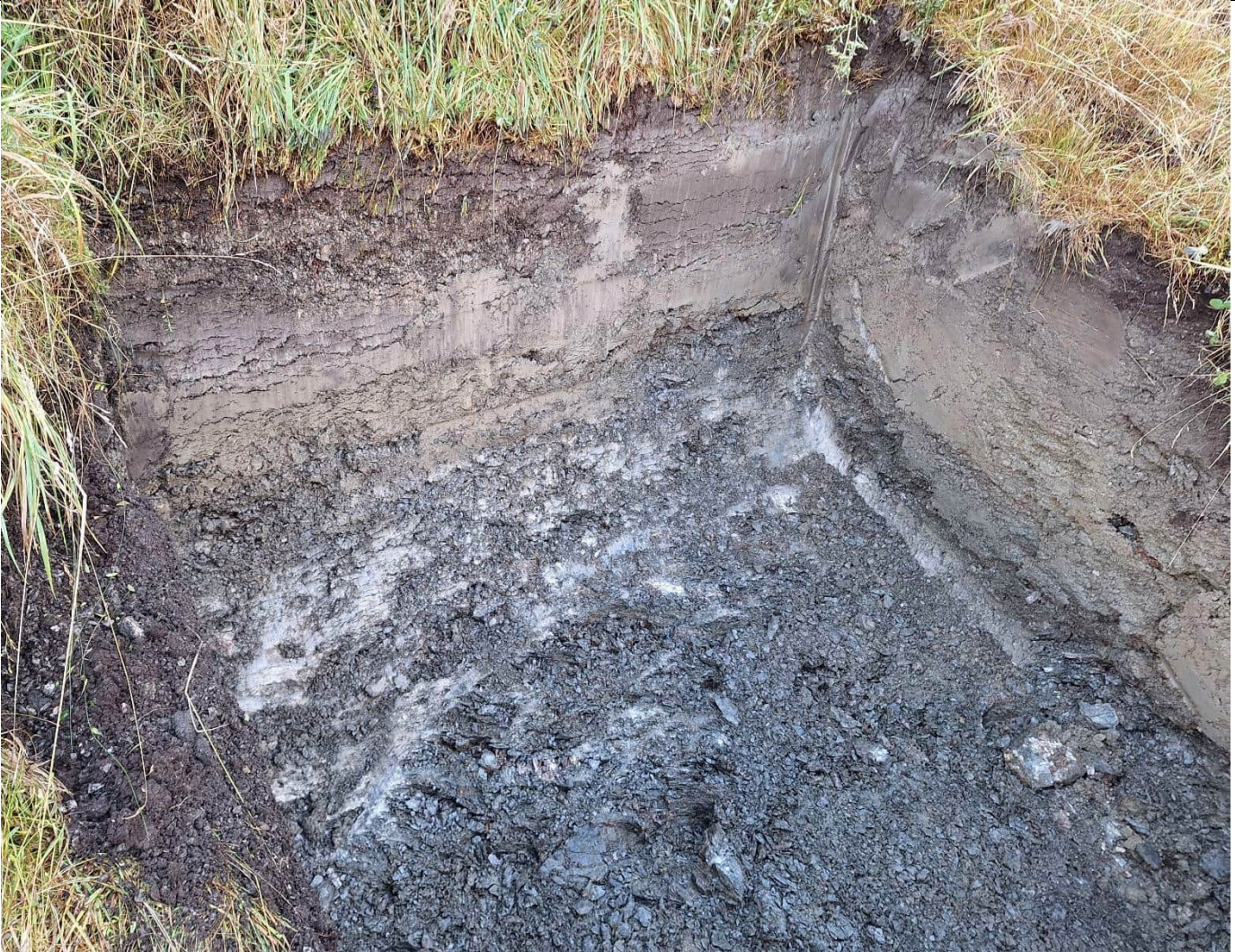
Testpit at completion. Max depth 1.3m
