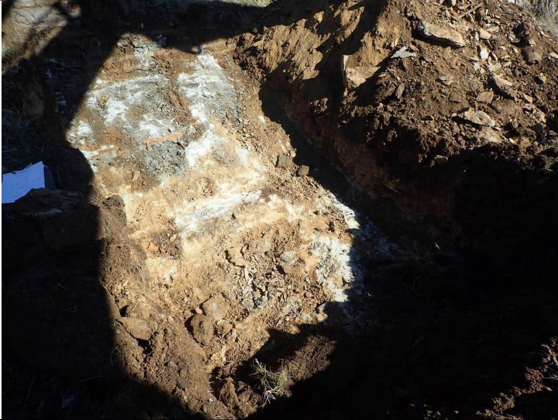
Testpit at completion. Max depth 1m
