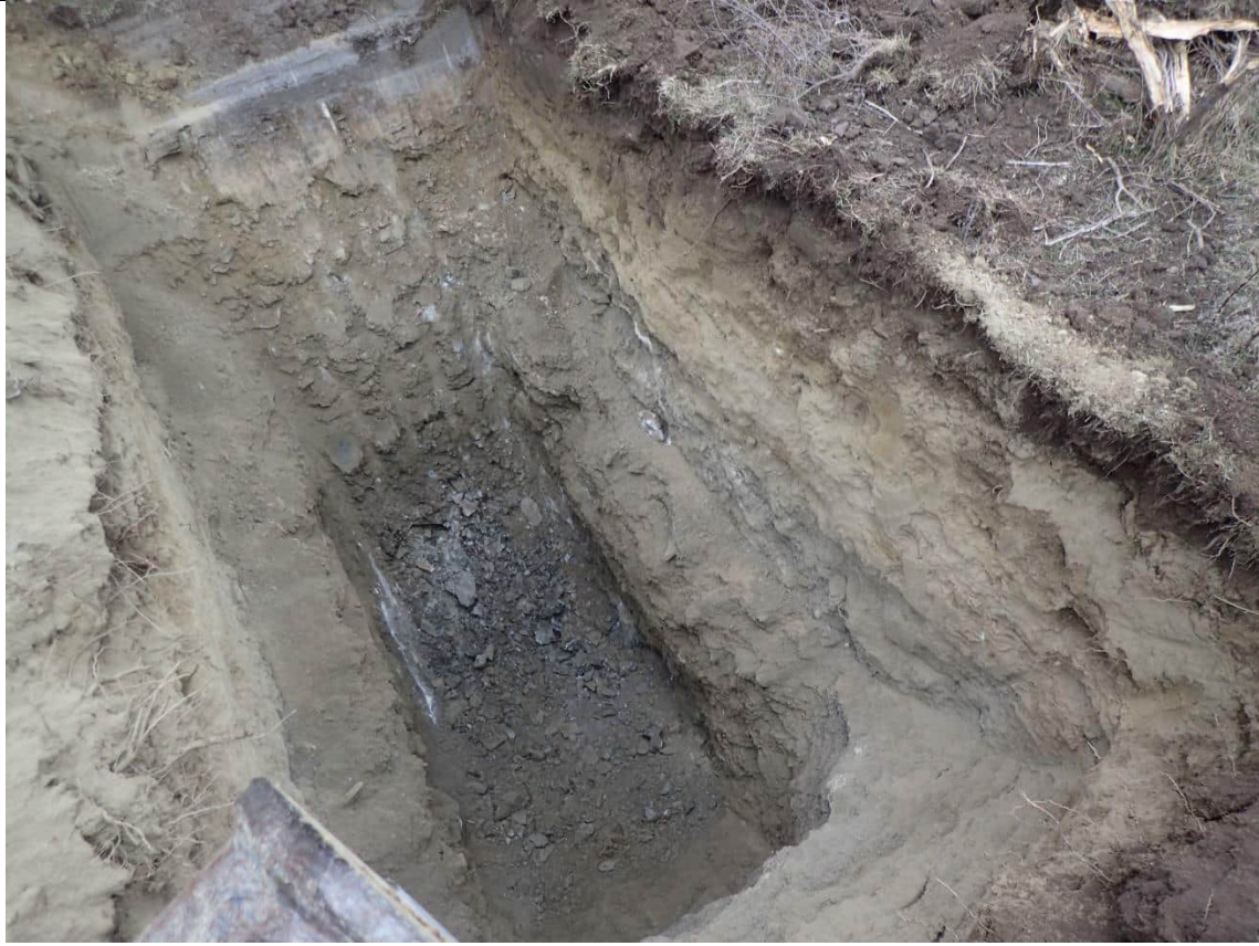
Testpit at completion. Max depth 3m
