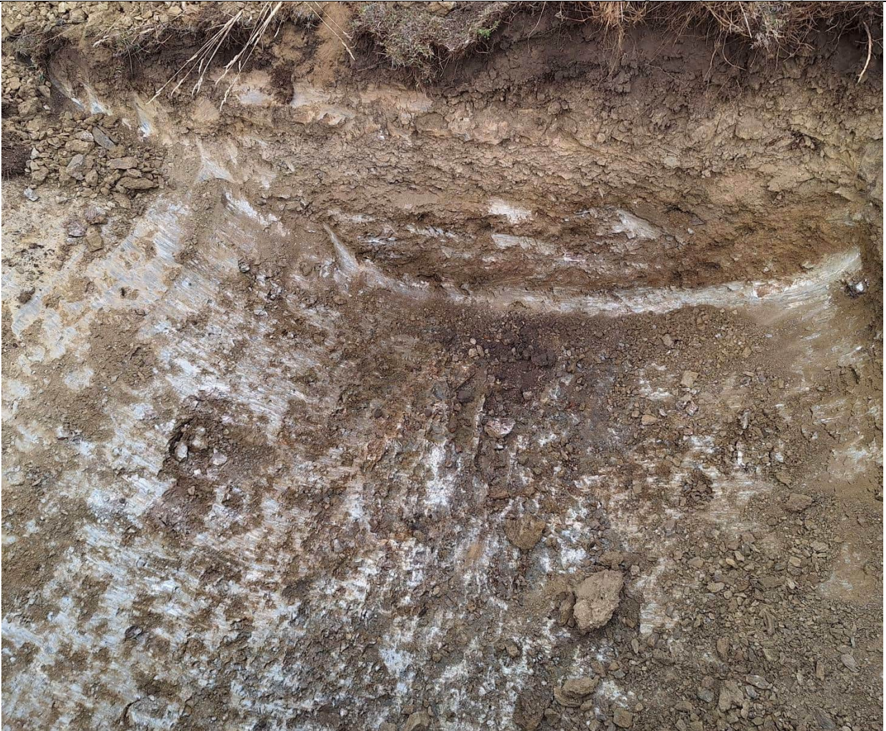
Testpit at completion. Max depth 0.9m
