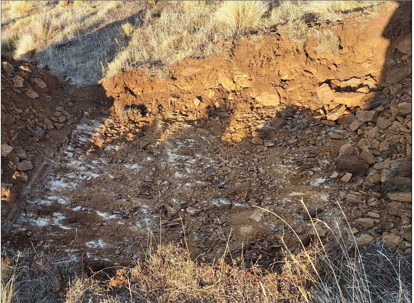
Testpit at completion. Max depth 0.4m
