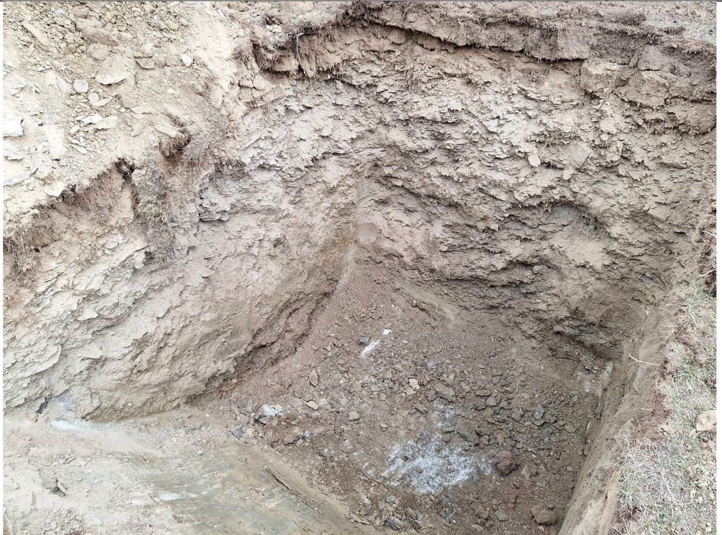
Testpit at completion. Max depth 2.5m
