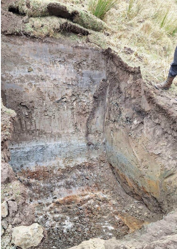
Testpit at completion. Max depth 1.8m
