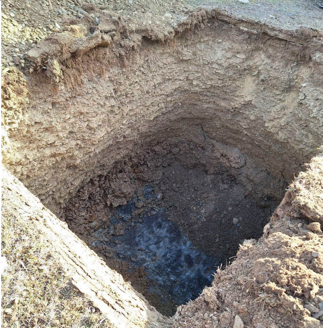
Testpit at completion. Max depth 2.9m
