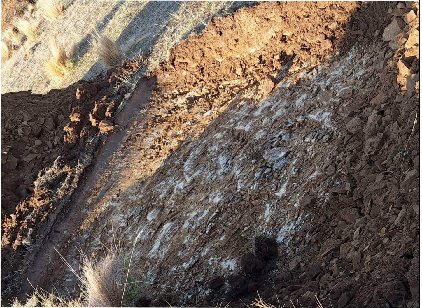
Testpit at completion. Max depth 0.3m
