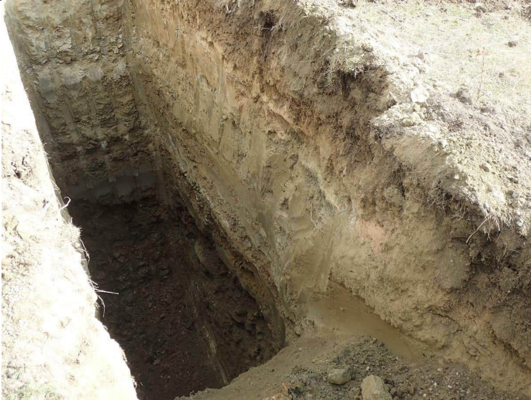
Testpit at completion. Max depth 5.5m
