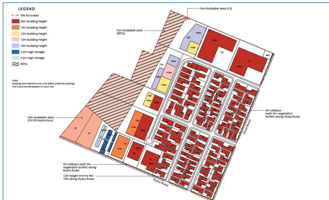
Figure 2: Building layout and height scheme
