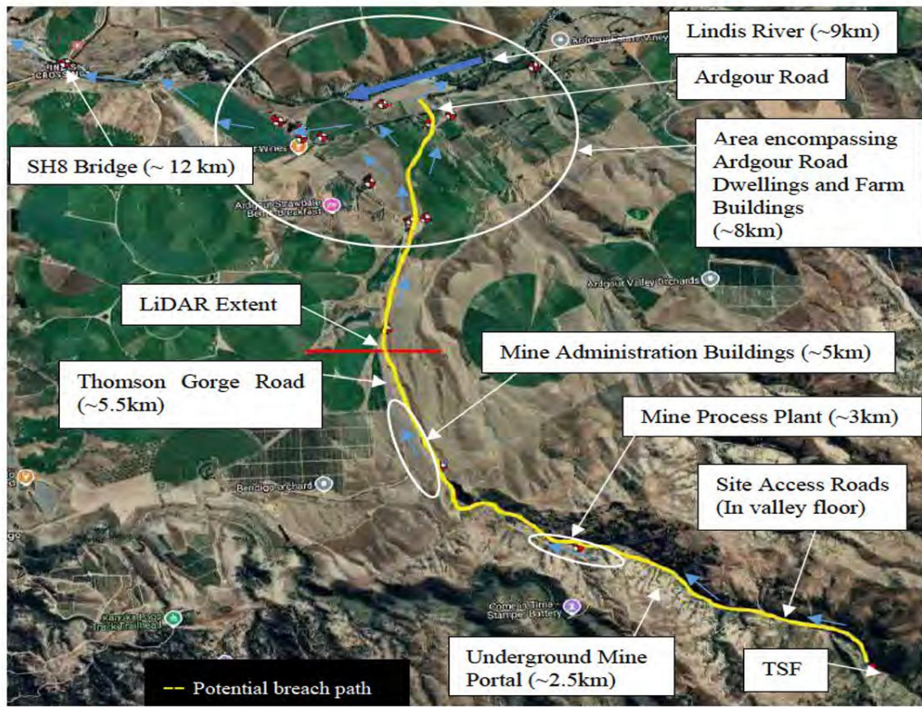
Figure 1: Potential breach flood path, items of interest and approximate distance downstream (Source: Google)
