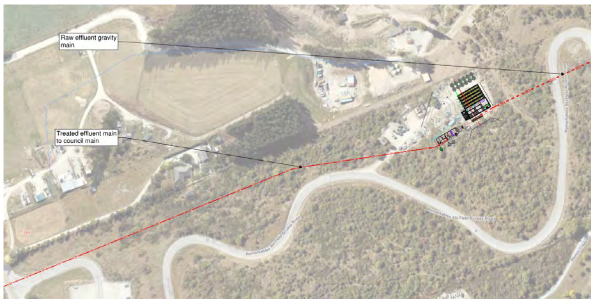
Figure 9. Treatment plant and treated effluent main crossing SH6.
