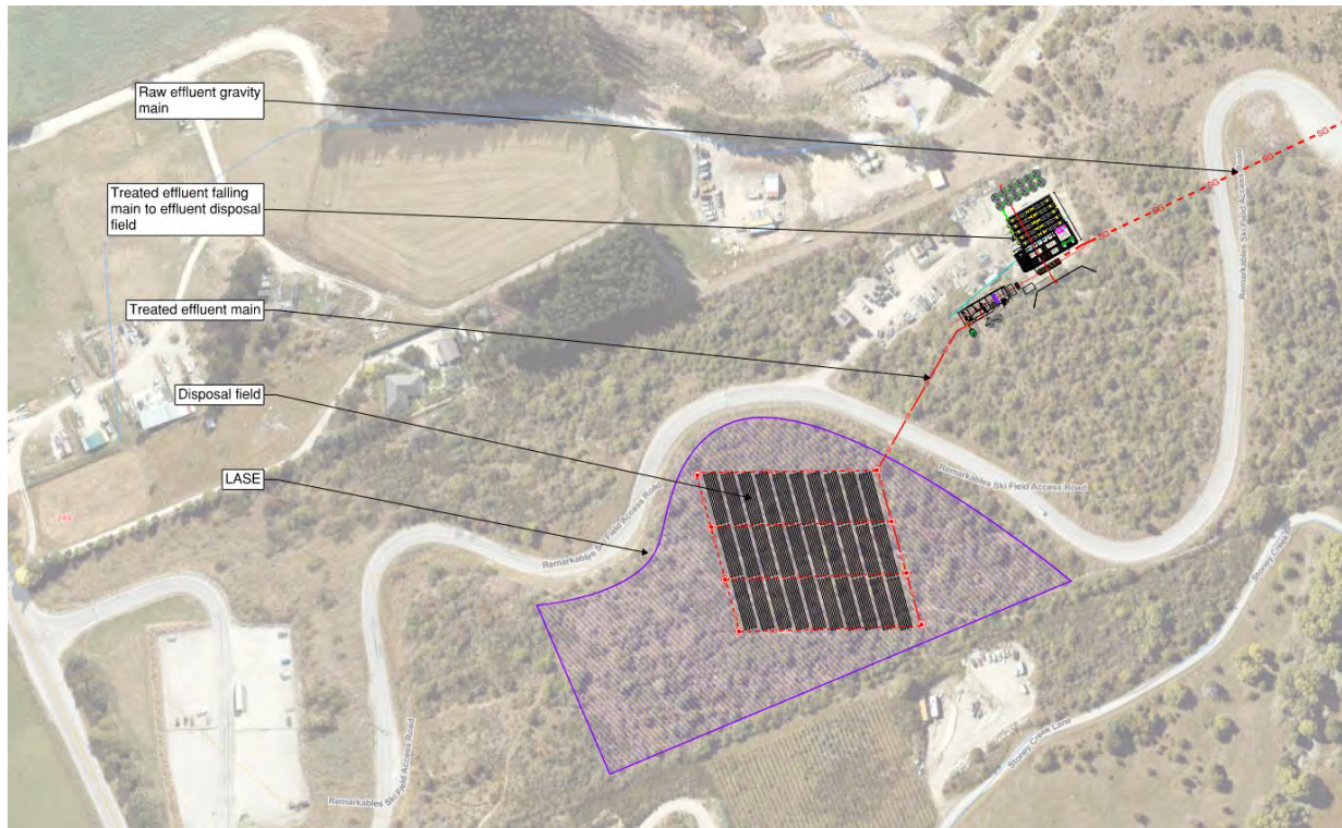
Figure 6. Treatment and disposal system in Trojan owned land.
