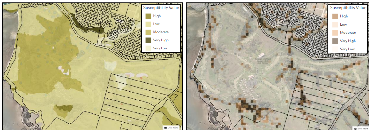
Figure 4.5: Auckland Council PC120 landslide hazard maps (Left: large-scale; Right: shallow instability)
