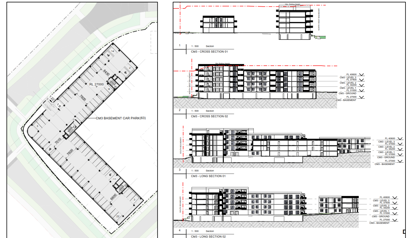
Figure 5.8: Concept plan and sections for the CM3 apartment basement (excerpt from drawings FC-CM3-105 & -200 rev A)
