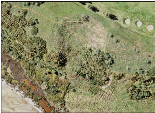
Figure 4.2: Historical landslide at the south-western edge of the proposed Coastal sub-precinct
