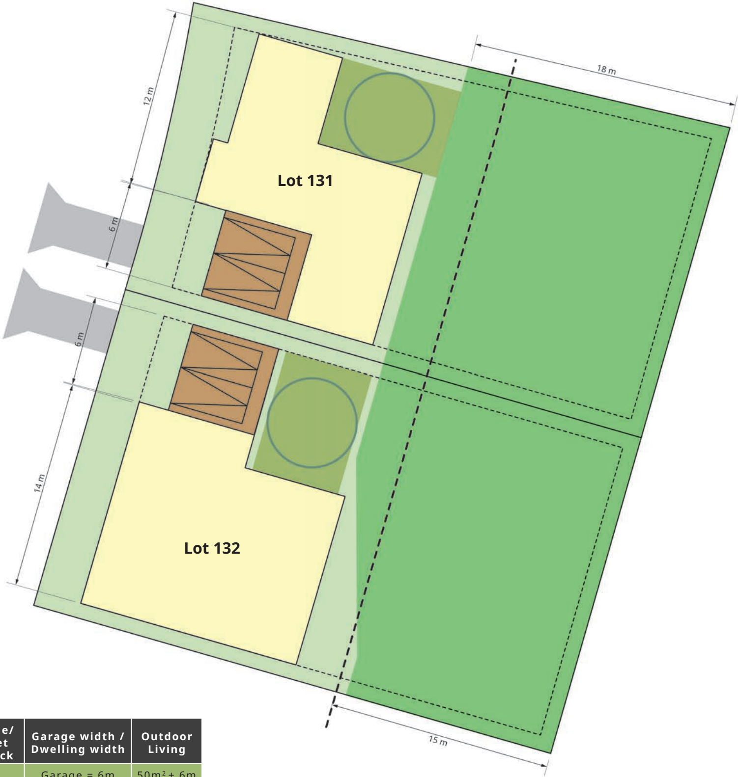
Figure 24 Indicative Layout for Lots 131 & 132 based on GRZ development controls
