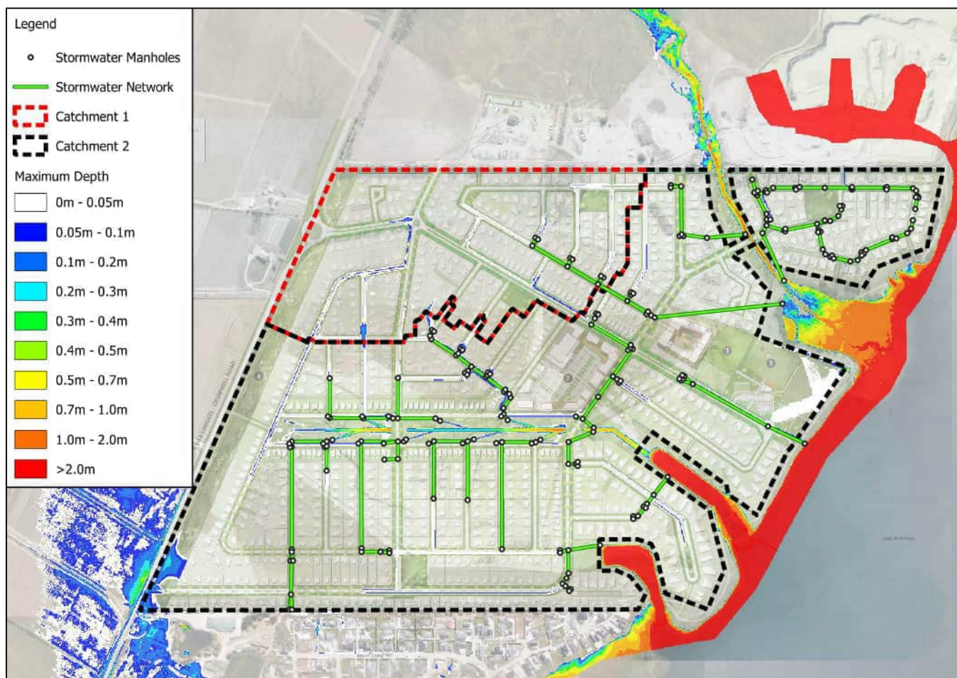
Figure 14: 5-year ARI internal flooding
