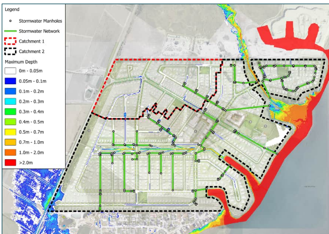
Figure 16: 10-year ARI internal flooding
