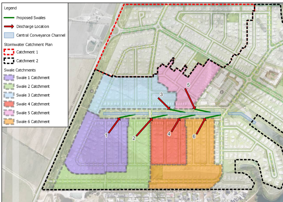
Figure 7: Swale Catchment Plan
