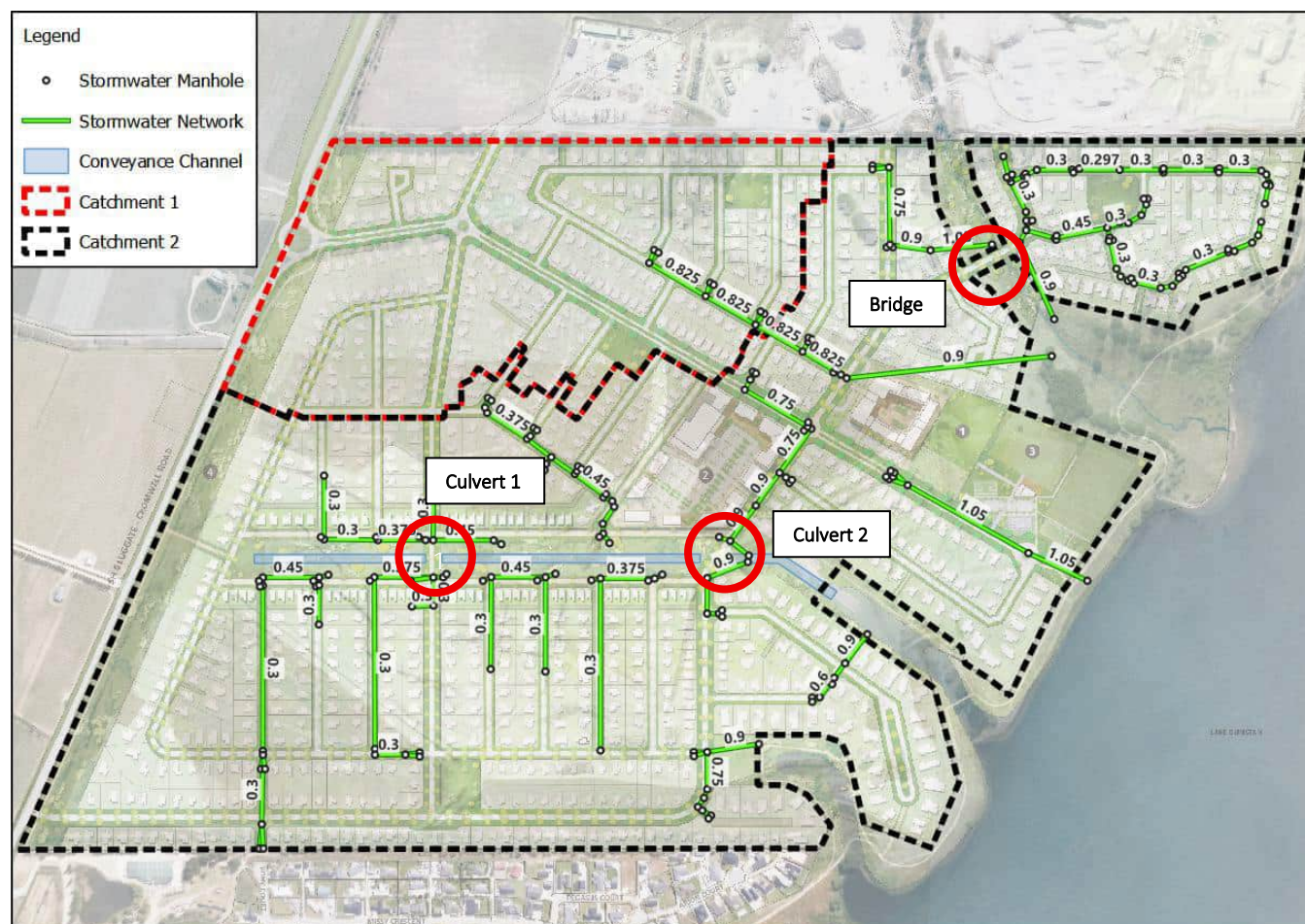
Figure 9: Preliminary stormwater pipe network
