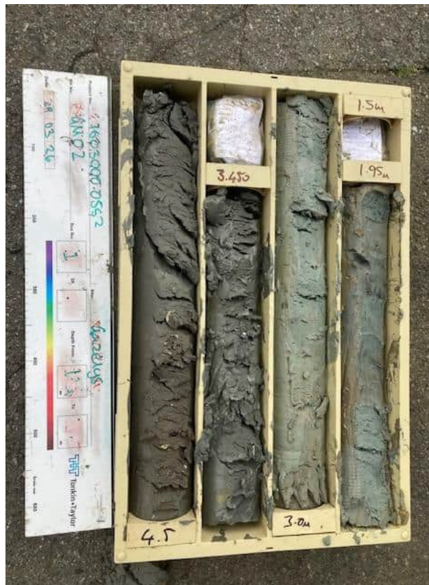
Photo 4:GM02 Soil Core 4.5 m to 7.5 m bgl 29-03-2026
