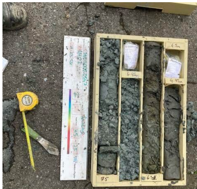
Photo 4:GM02 Soil Core 4.5 m to 7.5 m bgl 29-03-2026
