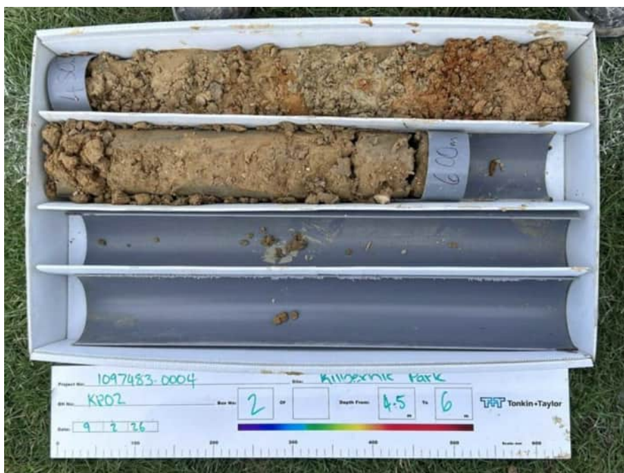
Photo 6: KP02 4.95 to 6.0 m depth 09-02-2026 (photo from T&T Borehole log KP02)
