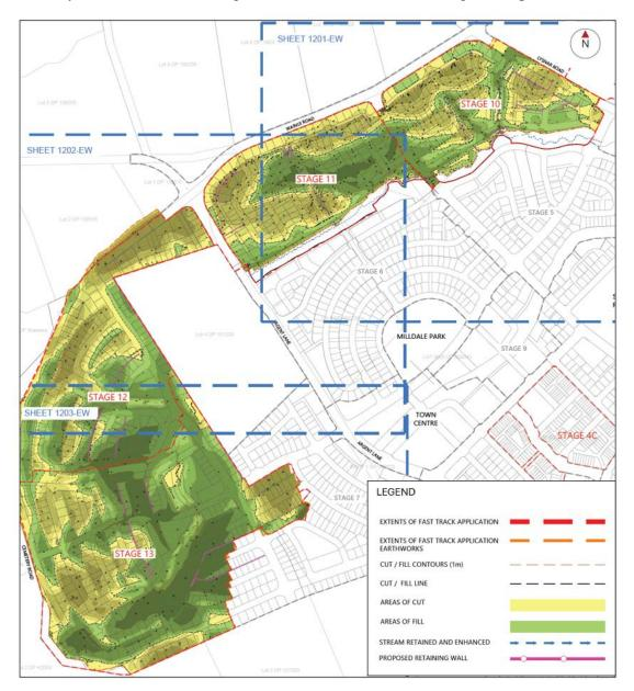
Figure 43. Overall Cut/ Fill plan for Stages 10-13 (source: Woods)
