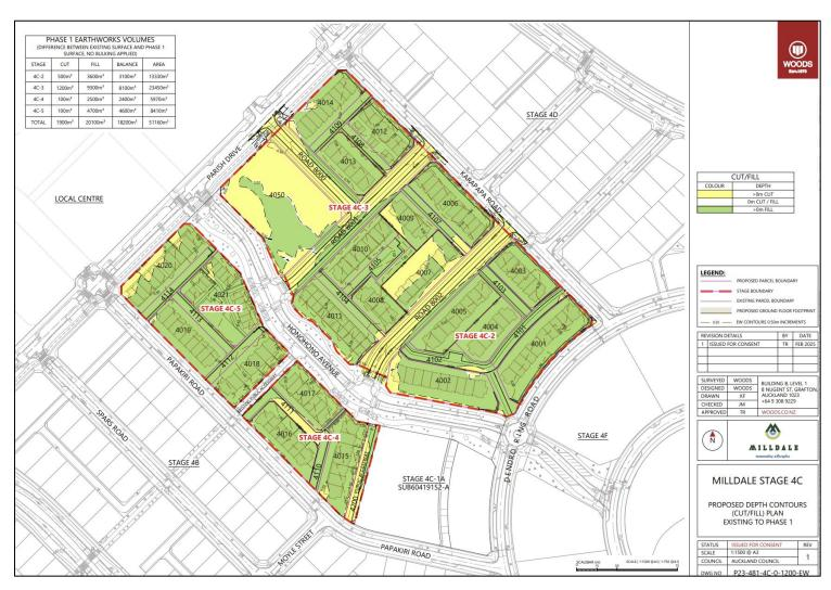
Figure 45. Cut fill plan of Stage 4C with Stage boundary outlined by red dashed line (source: Woods)
