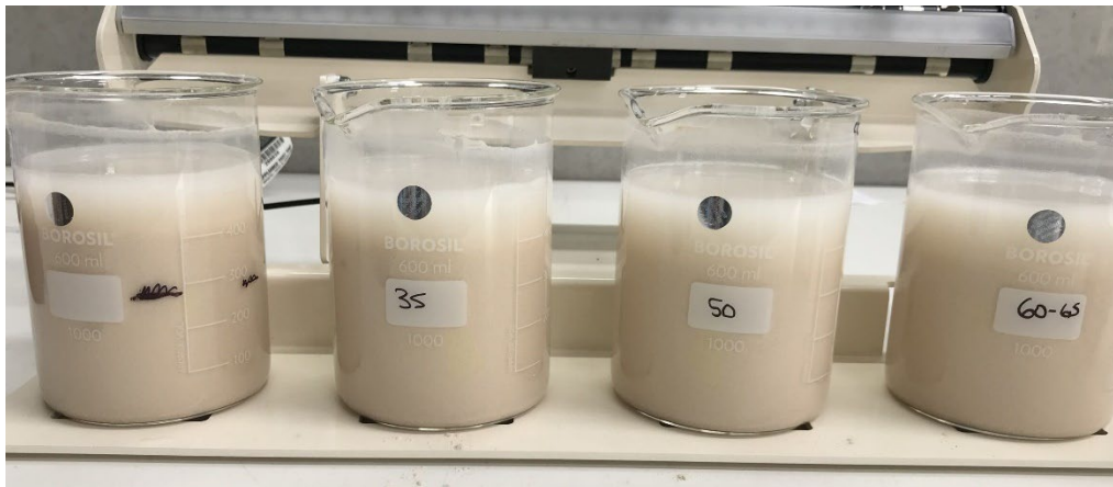
Figure 6 Farmguard Slurry 2 minutes after slaking finished, already settling out.
