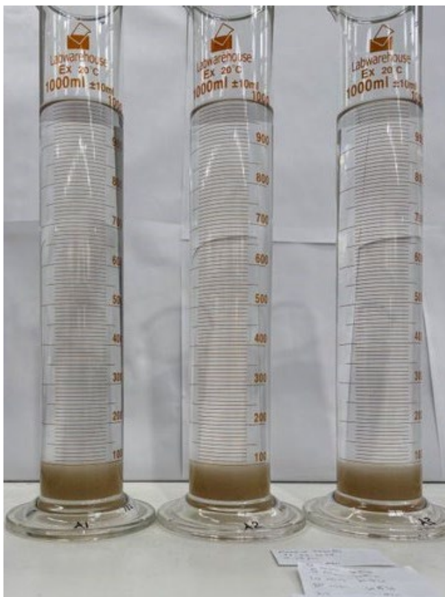
Figure 4 Makeup Water Testing - 30 mins settling
