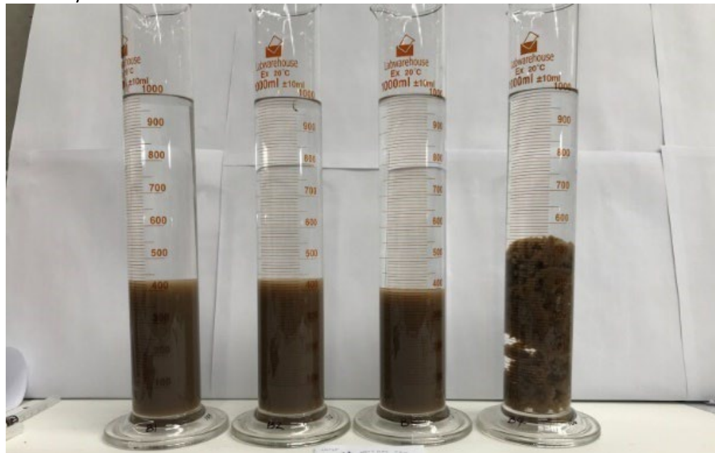
Figure 7 Sludge Thickening - S23 with Rheomax 1050
