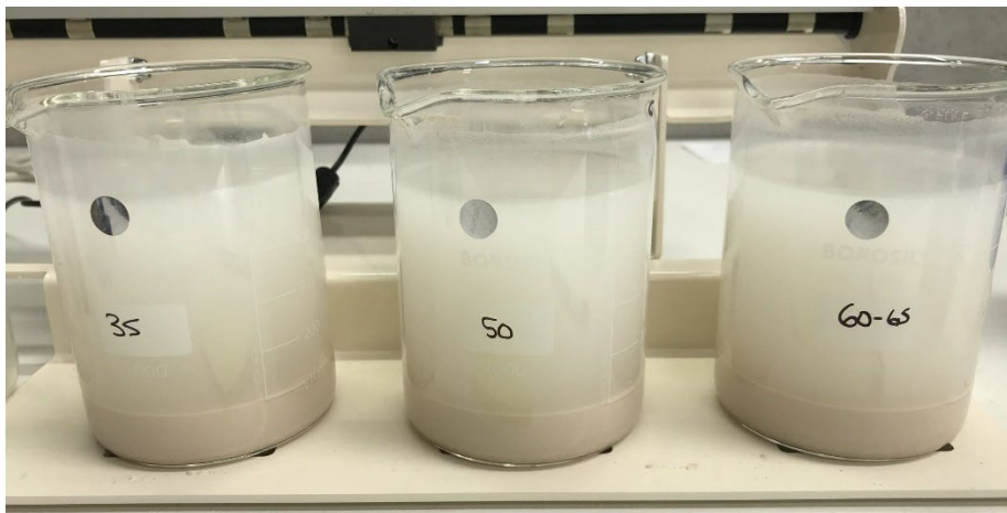
Figure 6 Farmguard Slurry 2 minutes after slaking finished, already settling out.
