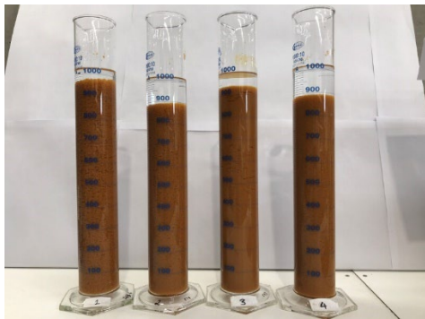
Figure 8 Sludge Thickening - S23 with Rheomax 1030
