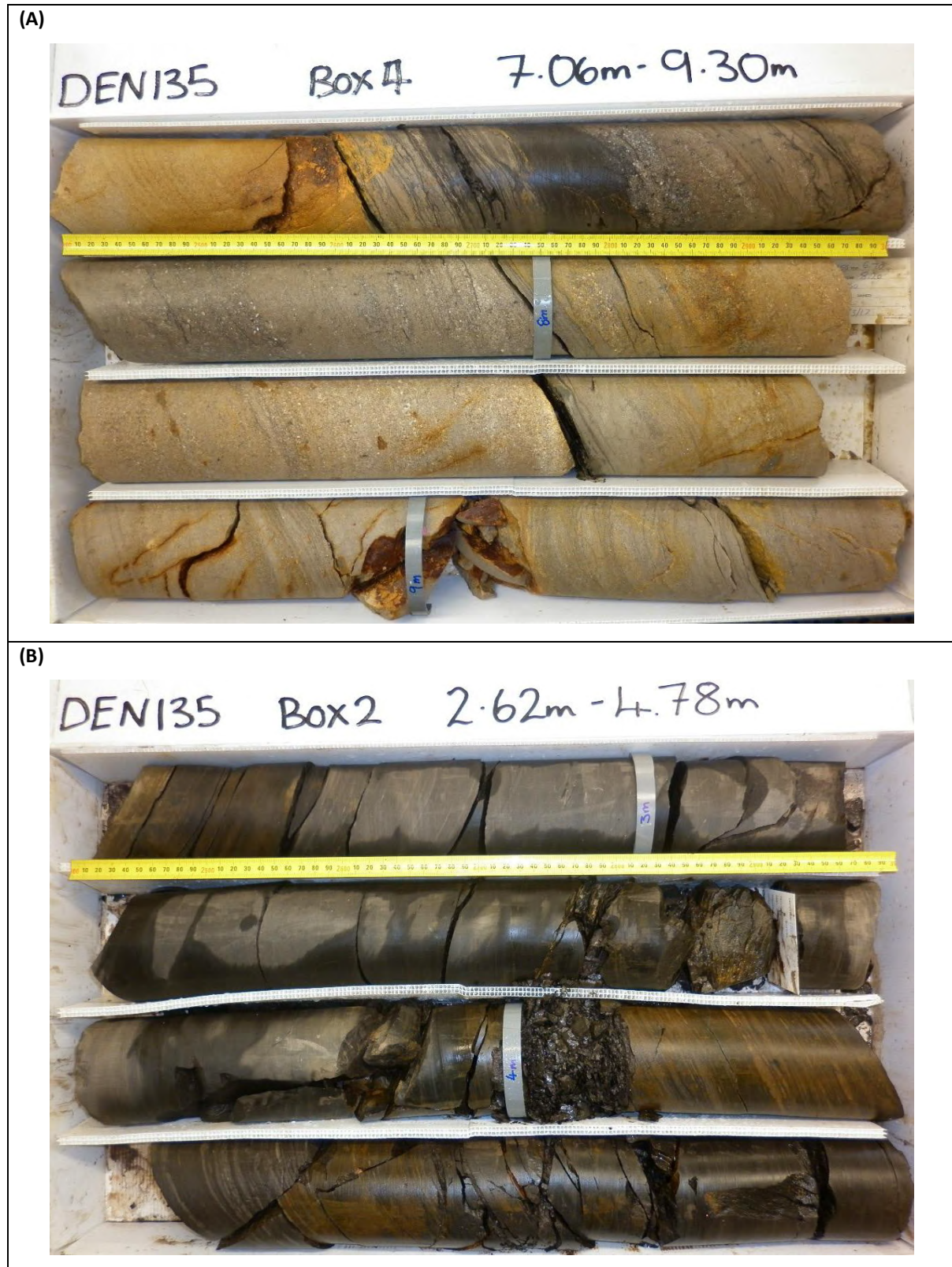
Figure 5. Drill core examples through Brunner Coal Measures sediments from bore hole DEN135. A) Fine – coarse grained sandstone, representative of the typical overburden found at the site. B) Fine sandstone and mudstone with minor carbonations bands, less frequent at the site.
