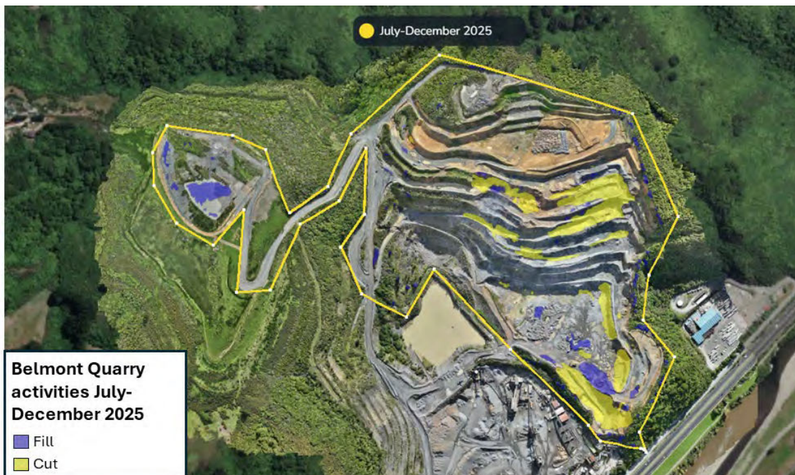
Figure 4: Location of Cut and Fill Activities at Belmont Quarry between July to December 2025
