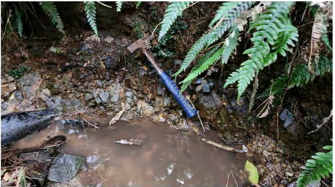
Photograph 6: Highly weathered Greywacke exposed in the stream channel. Gully alluvium was also present in form of gravel and cobbles within a matrix of clay and silt at location Bx06 [western gully].
