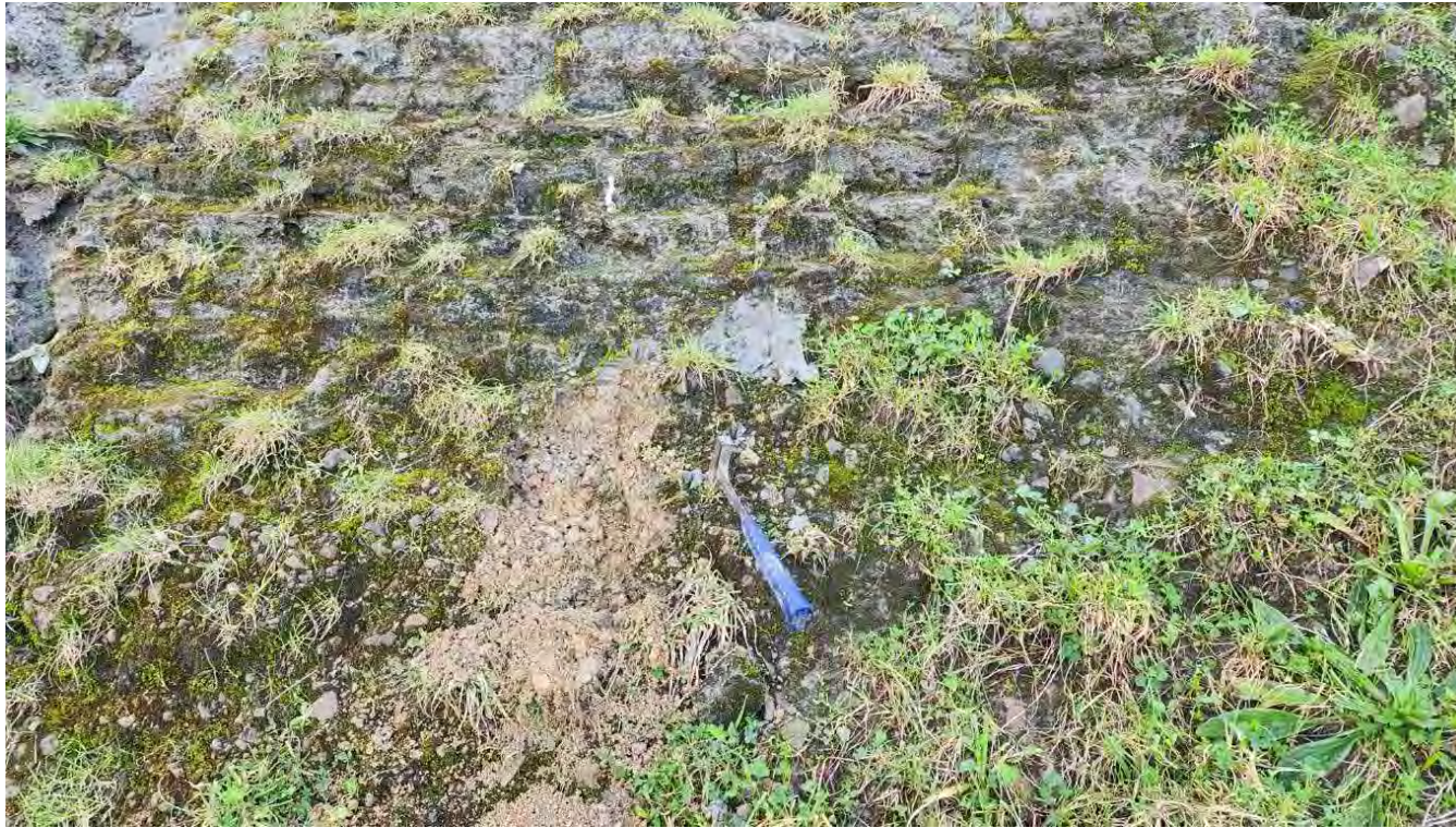
BQ01: Contact between process fines and underlying historic quarry backfill.
