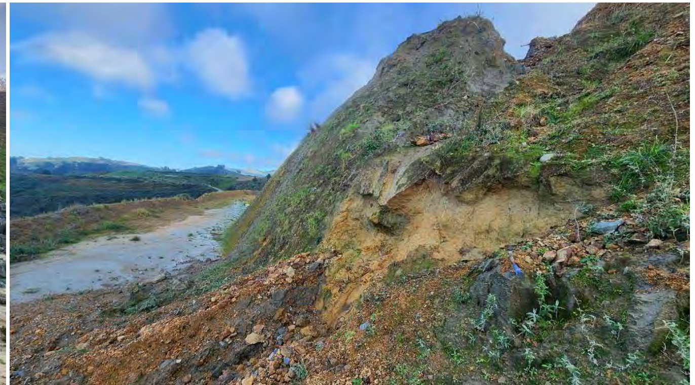
BQ11: Process fines overlying residual soils and weathered greywacke rock.
