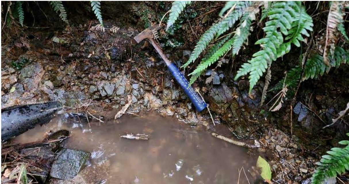
Figure 5-1: Highly weathered greywacke rock exposure in Western Gully floor at Bx06.
