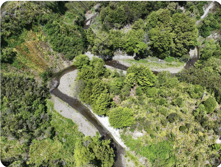
Typical deeply incised character with depositional gravel bars on insides of meanders and steep cuts on the outsides. Drone Image provided by Applicant.
