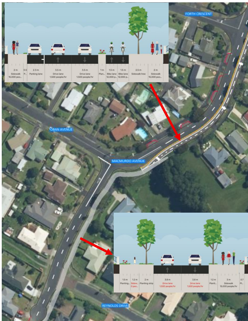
Figure 30: Indicative Alignment and Cross-section of MacMurdo Ave
