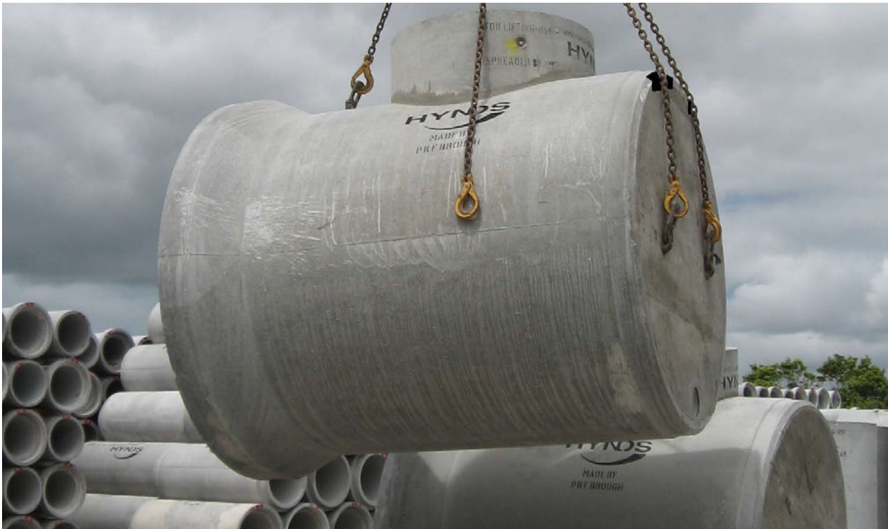
FIG. 6 Point lift of typical plugged end pipe
