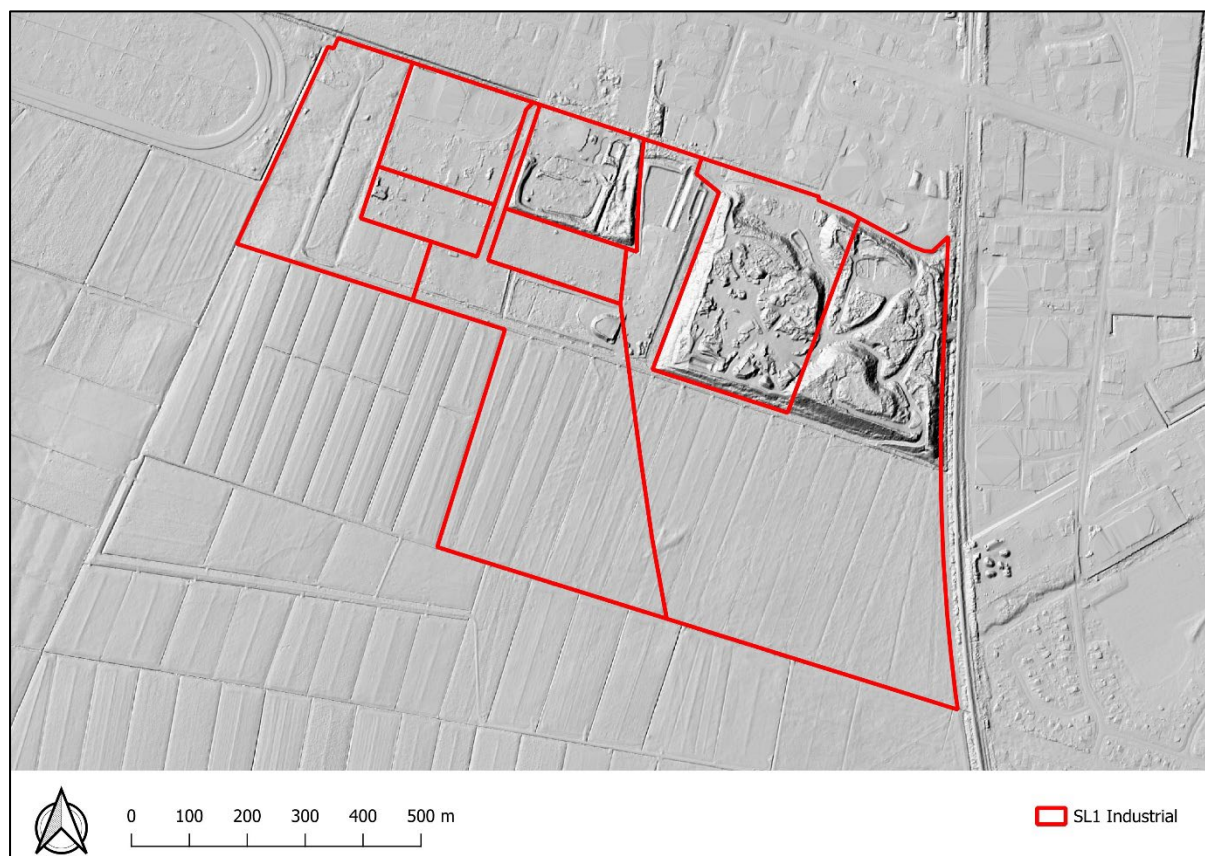
Figure 15. Lidar derived hillshade model from DEM data taken in 2023 that shows the Site as mostly flat with some lower hills to the north (Source: LINZ).
