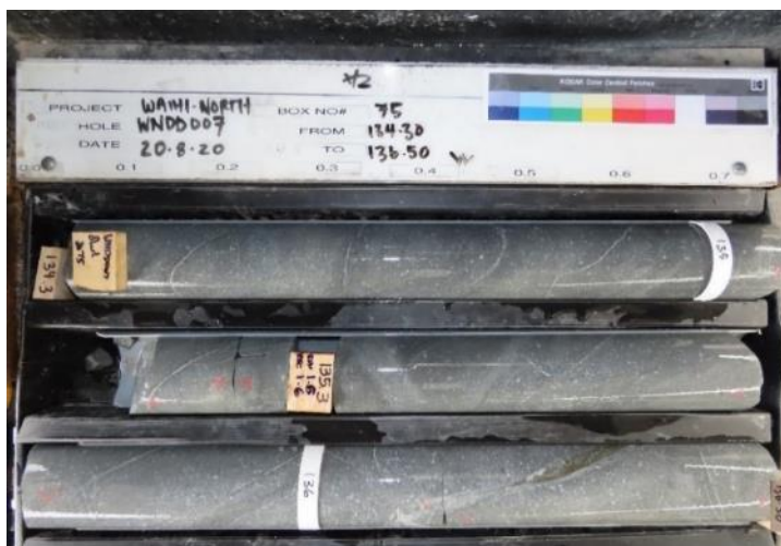
Figure 10: Porphyritic andesite recovered from WNDD007.
