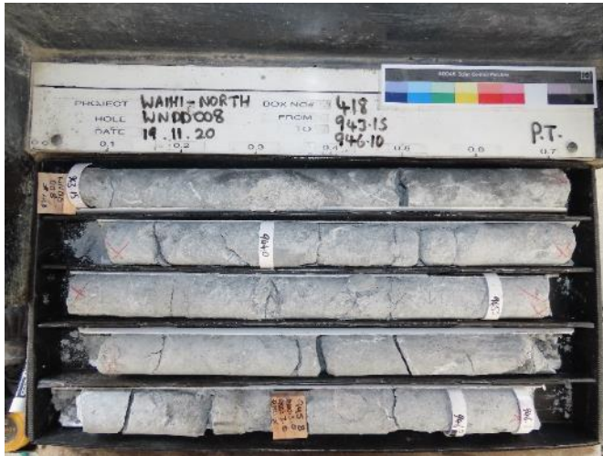
Figure 13: Lapilli tuff recovered from WNDD008.
