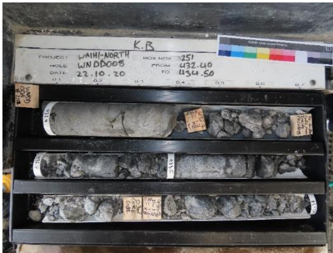
Figure 15: Lapilli tuff recovered as gravel from WNDD008.
