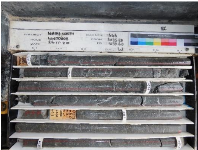
Figure 14: Porphyritic andesite recovered from WNDD008.
