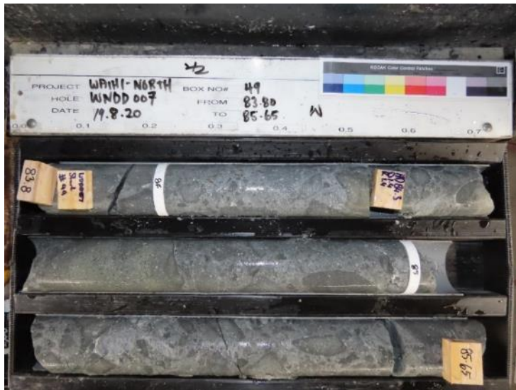
Figure 9: Autoclastic breccia andesite recovered from WNDD007.
