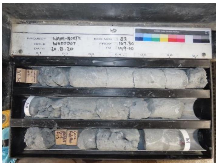
Figure 11: Clay altered sample from WNDD007.
