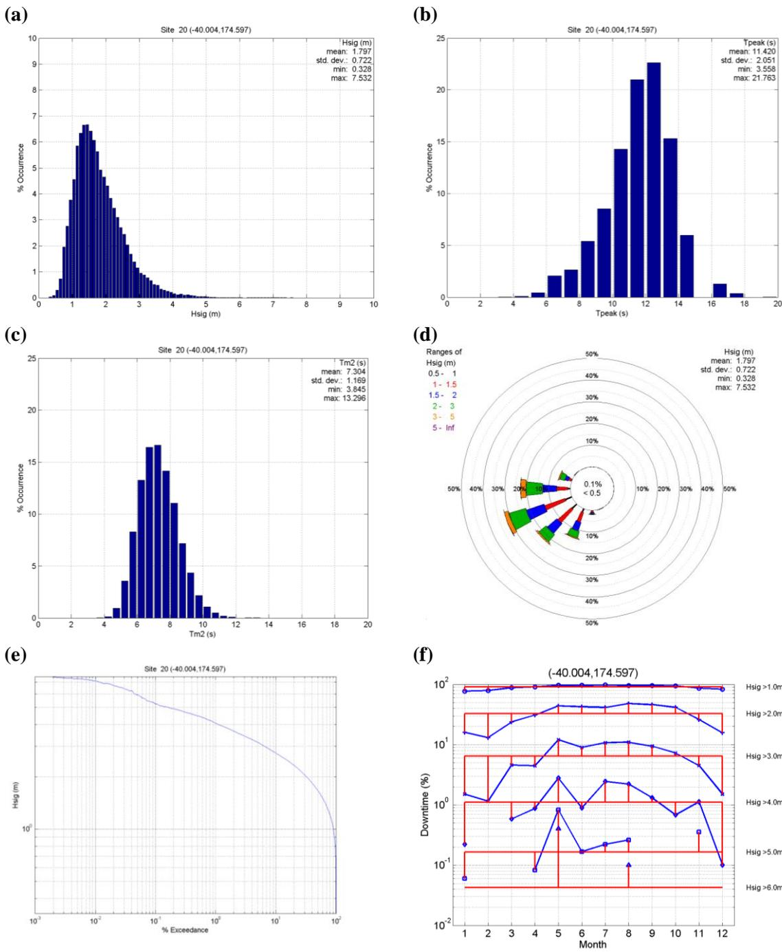
**Figure 2.11. Occurrence statistics for site 20 at (40.004°S, 174.597°E) from the full 1979-1998 hindcast. The first three plots show percentage occurrence for (a) significant wave height, (b) peak wave period, and (c) mean wave period (second moment). Also shown are (d) the wave rose, (e) the wave height exceedance distribution, and (f) “downtime”, i.e. the percentage of time that given significant wave height thresholds are exceeded for each month.**
