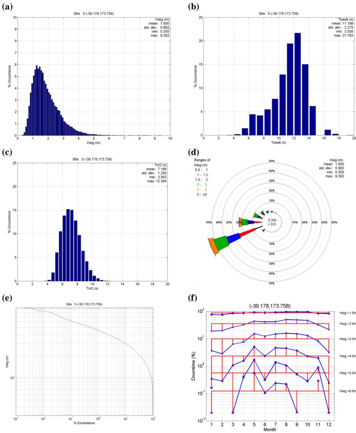
**Figure 2.5.** Occurrence statistics for site 5 at (39.176°S, 173.758°E) from the full 1979-1998 hindcast. The first three plots show percentage occurrence for (a) significant wave height, (b) peak wave period, and (c) mean wave period (second moment). Also shown are (d) the wave rose, (e) the wave height exceedance distribution, and (f) “downtime”, i.e. the percentage of time that given significant wave height thresholds are exceeded for each month.
