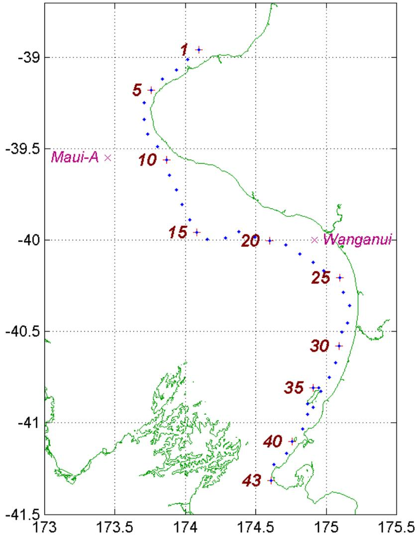
**Figure 2.1.** Wave hindcast output locations on the 50 m isobath, with every 5<sup>th</sup> location numbered. The locations of wave buoys (Maui-A, Wanganui) used for verification are also marked.
