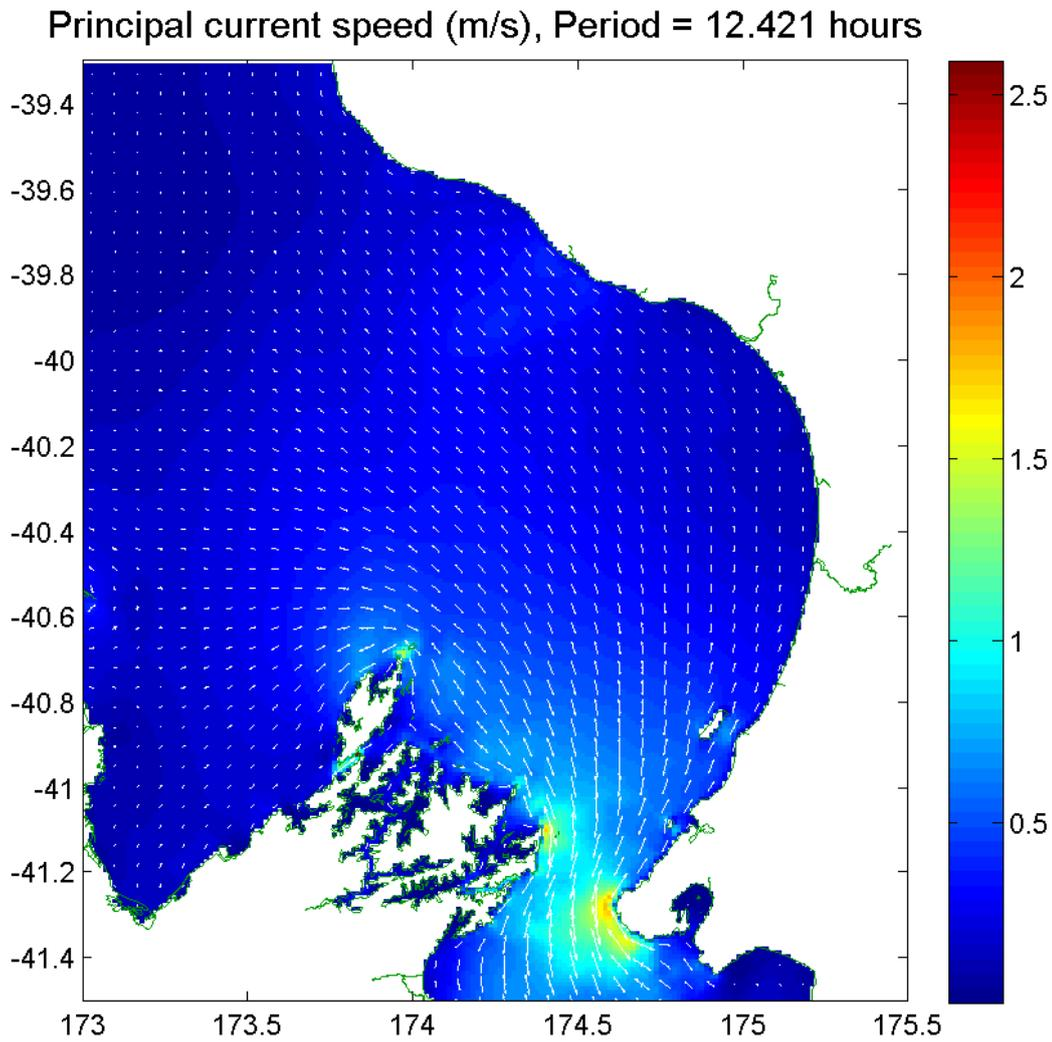
**Figure 2.21(a).** Peak velocity of the M<sub>2</sub> component of the tidal current. The maximum speed is shown by the colour scale, while maximum and minimum velocity vectors are shown by the longer and shorter of the crossed arrows, respectively.
