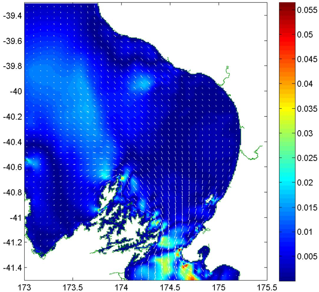
**Figure 2.23(b). Minimum velocity of the N<sub>2</sub> component of the tidal current. The minimum speed is shown by the colour scale, while maximum and minimum velocity vectors are shown by the longer and shorter of the crossed arrows, respectively.**
