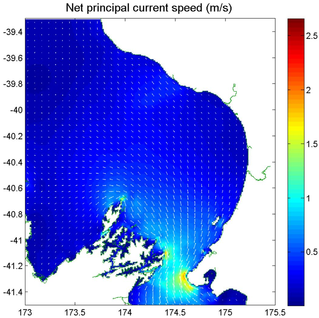
**Figure 2.24(a). Peak velocity of the net tidal current. The maximum speed is shown by the colour scale, while maximum and minimum velocity vectors are shown by the longer and shorter of the crossed arrows, respectively.**
