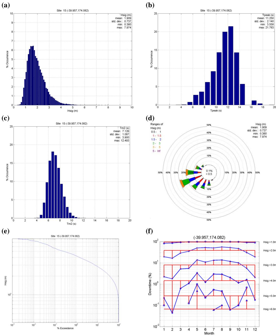
**Figure 2.9.** Occurrence statistics for site 15 at (39.957°S, 174.082°E) from the full 1979-1998 hindcast. The first three plots show percentage occurrence for (a) significant wave height, (b) peak wave period, and (c) mean wave period (second moment). Also shown are (d) the wave rose, (e) the wave height exceedance distribution, and (f) “downtime”, i.e. the percentage of time that given significant wave height thresholds are exceeded for each month.
