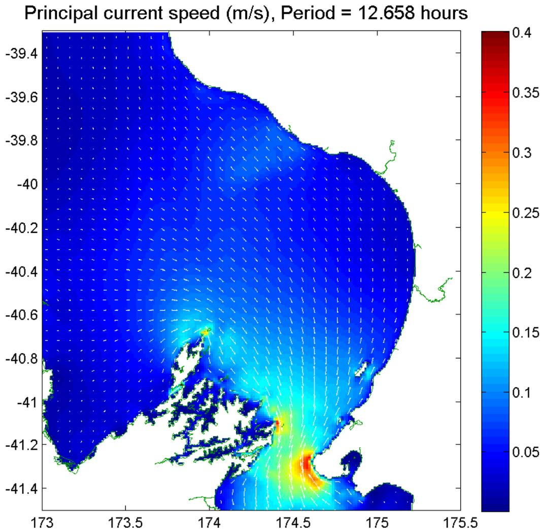
**Figure 2.23(a).** Peak velocity of the  $N_2$  component of the tidal current. The maximum speed is shown by the colour scale, while maximum and minimum velocity vectors are shown by the longer and shorter of the crossed arrows, respectively.
