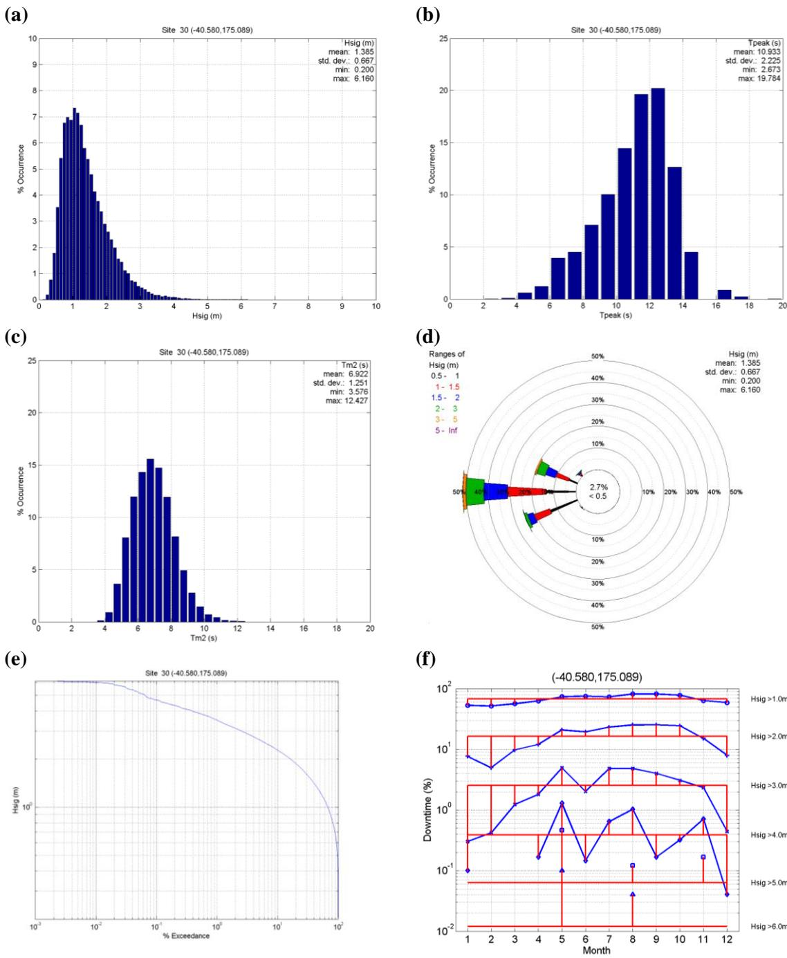
**Figure 2.15.** Occurrence statistics for site 30 at (40.580°S, 175.089°E) from the full 1979-1998 hindcast. The first three plots show percentage occurrence for (a) significant wave height, (b) peak wave period, and (c) mean wave period (second moment). Also shown are (d) the wave rose, (e) the wave height exceedance distribution, and (f) “downtime”, i.e. the percentage of time that given significant wave height thresholds are exceeded for each month.
