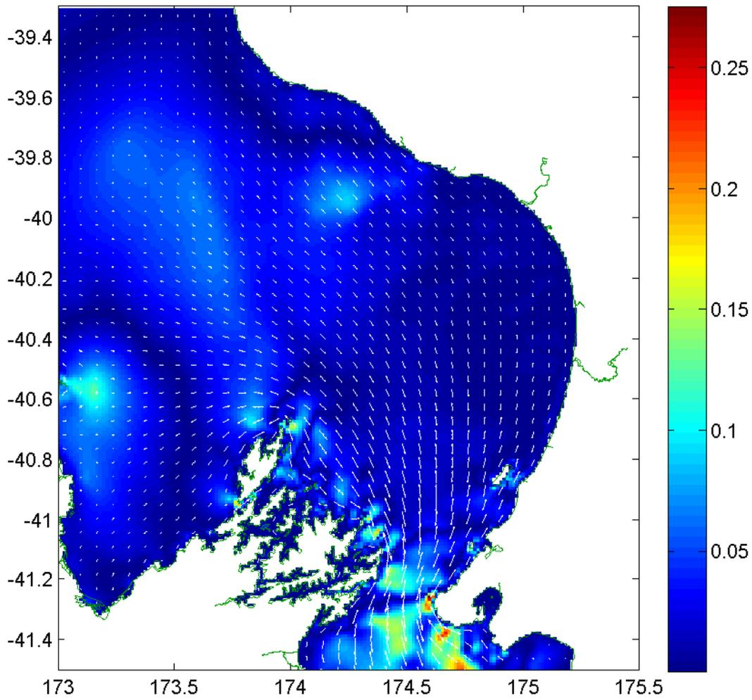
**Figure 2.21(b). Minimum velocity of the M<sub>2</sub> component of the tidal current. The minimum speed is shown by the colour, while maximum and minimum velocity vectors are shown by the longer and shorter of the crossed arrows, respectively.**
