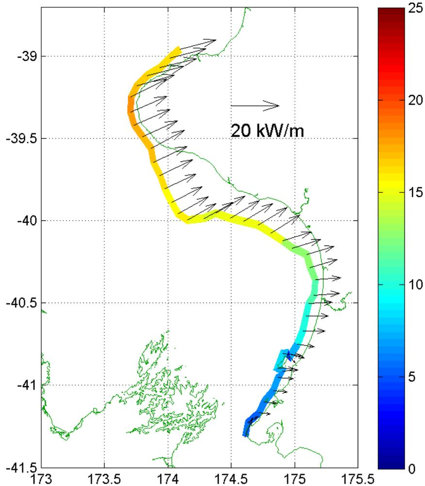
**Figure 2.4.** Spatial distribution along the 50 m isobath of mean wave energy flux, averaged over the full 20-year hindcast record. The colour scale shows the mean of the magnitude of the energy flux, while the arrows show the vector averaged flux.
