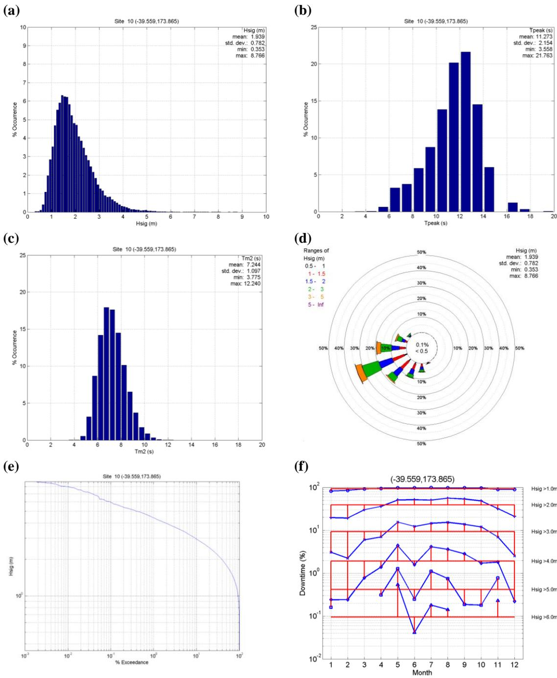
**Figure 2.7.** Occurrence statistics for site 10 at (39.559°S, 173.865°E) from the full 1979-1998 hindcast. The first three plots show percentage occurrence for (a) significant wave height, (b) peak wave period, and (c) mean wave period (second moment). Also shown are (d) the wave rose, (e) the wave height exceedance distribution, and (f) “downtime”, i.e. the percentage of time that given significant wave height thresholds are exceeded for each month.
