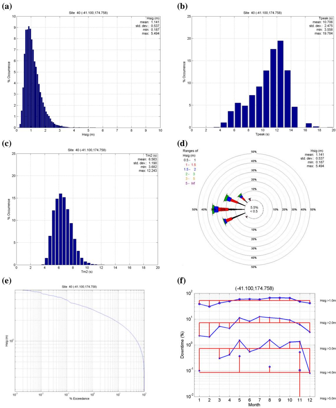
**Figure 2.19.** Occurrence statistics for site 40 at (41.100°S, 174.758°E) from the full 1979-1998 hindcast. The first three plots show percentage occurrence for (a) significant wave height, (b) peak wave period, and (c) mean wave period (second moment). Also shown are (d) the wave rose, (e) the wave height exceedance distribution, and (f) “downtime”, i.e. the percentage of time that given significant wave height thresholds are exceeded for each month.
