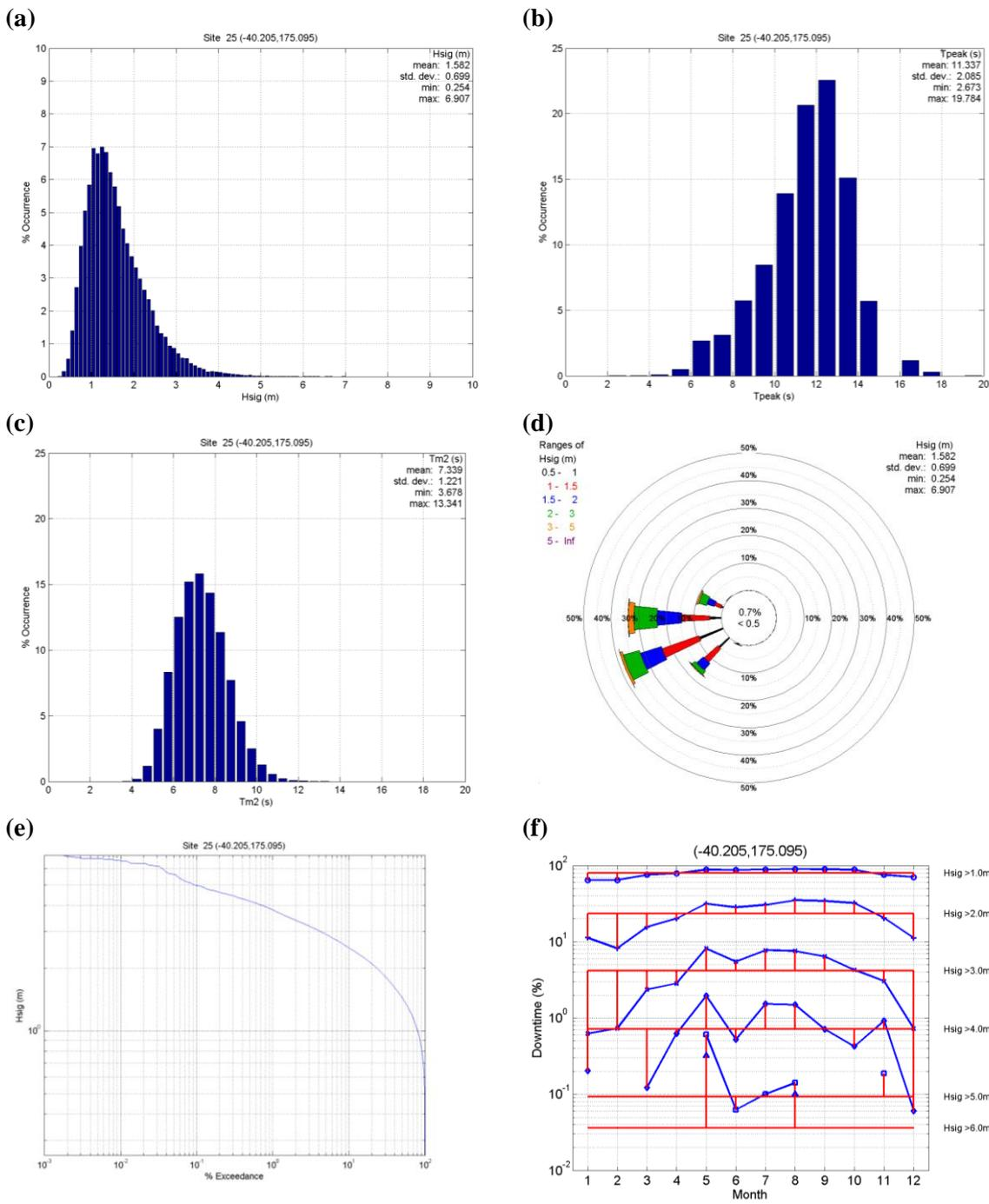
**Figure 2.13.** Occurrence statistics for site 25 at (40.205°S, 175.095°E) from the full 1979-1998 hindcast. The first three plots show percentage occurrence for (a) significant wave height, (b) peak wave period, and (c) mean wave period (second moment). Also shown are (d) the wave rose, (e) the wave height exceedance distribution, and (f) “downtime”, i.e. the percentage of time that given significant wave height thresholds are exceeded for each month.
