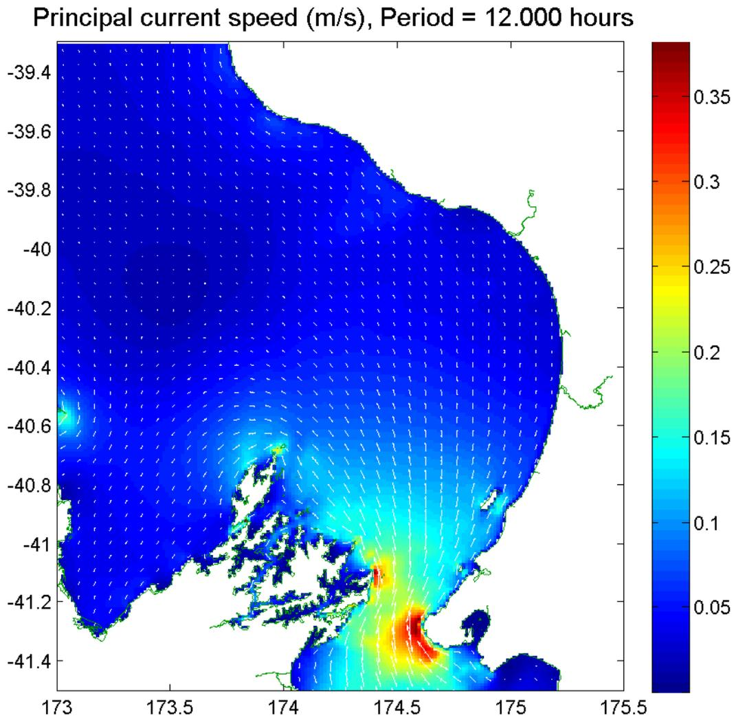
**Figure 2.22(a).** Peak velocity of the S<sub>2</sub> component of the tidal current. The maximum speed is shown by the colour scale, while maximum and minimum velocity vectors are shown by the longer and shorter of the crossed arrows, respectively.
