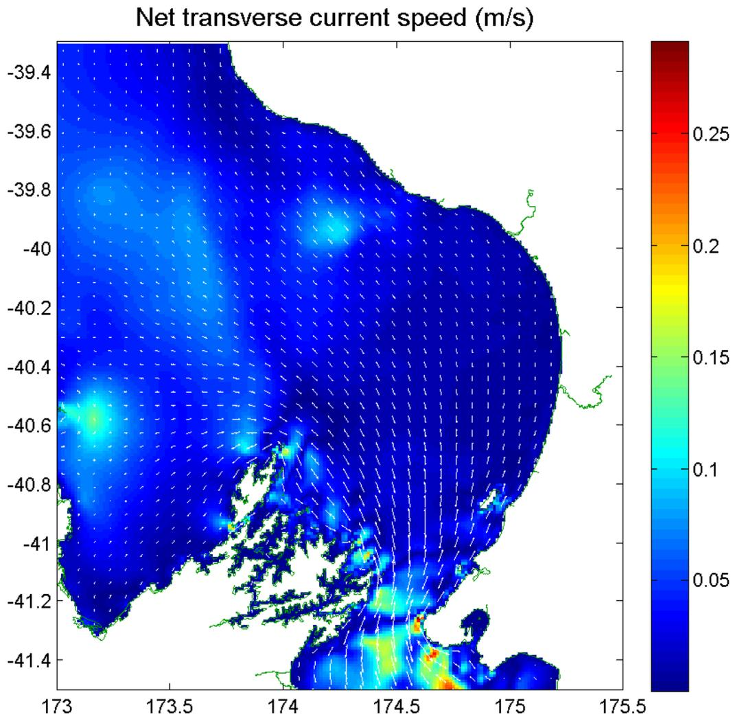
**Figure 2.24(b). Minimum velocity of the net tidal current. The minimum speed is shown by the colour scale, while maximum and minimum velocity vectors are shown by the longer and shorter of the crossed arrows, respectively.**
