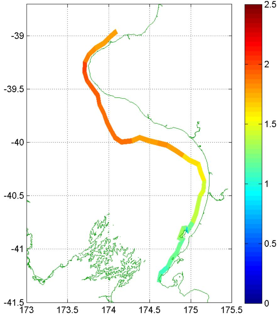
**Figure 2.3.** Spatial distribution along the 50 m isobath of mean significant wave height, averaged over the full 20-year hindcast record.
