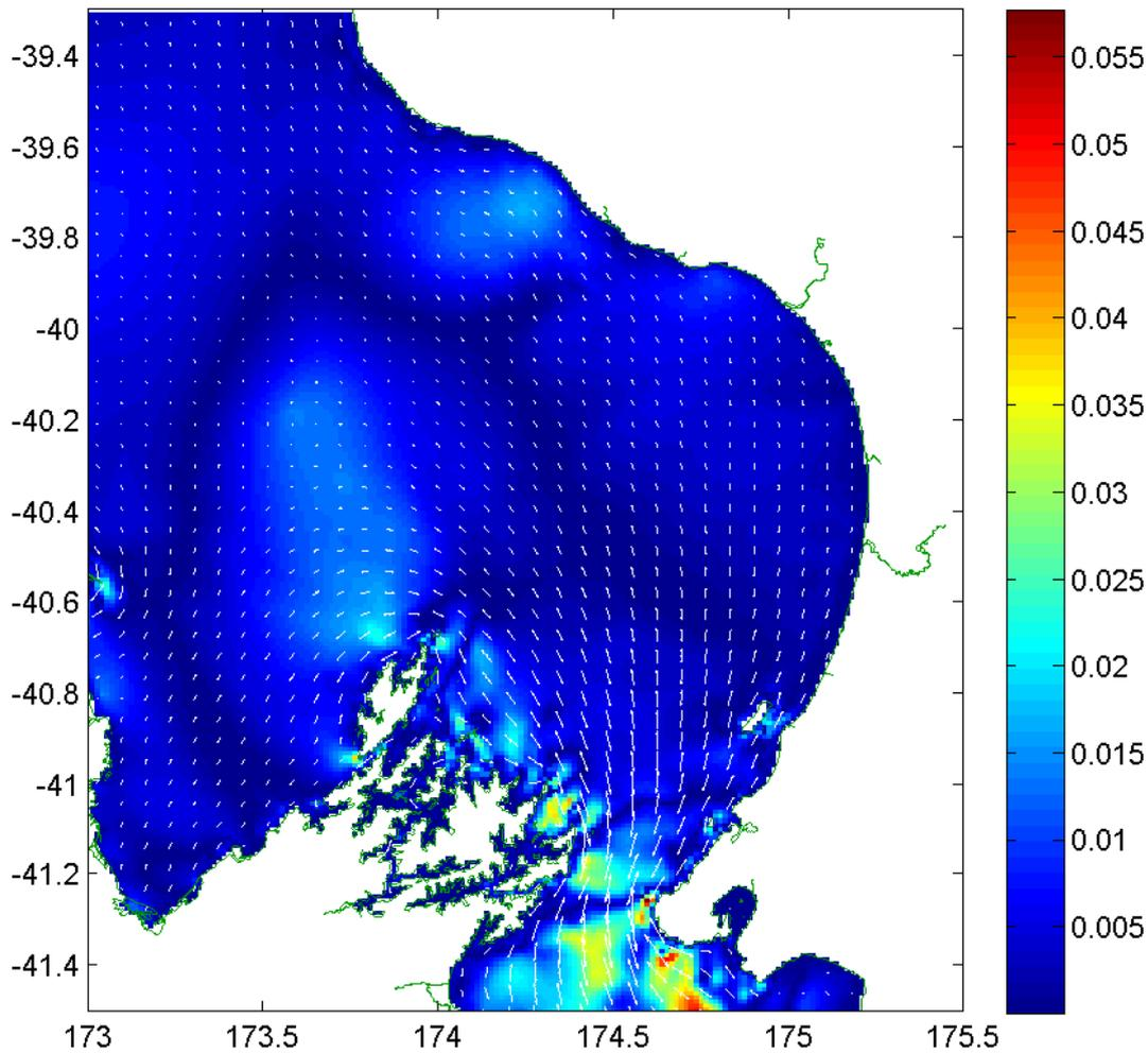
**Figure 2.22(b). Minimum velocity of the S<sub>2</sub> component of the tidal current. The minimum speed is shown by the colour scale, while maximum and minimum velocity vectors are shown by the longer and shorter of the crossed arrows, respectively.**
