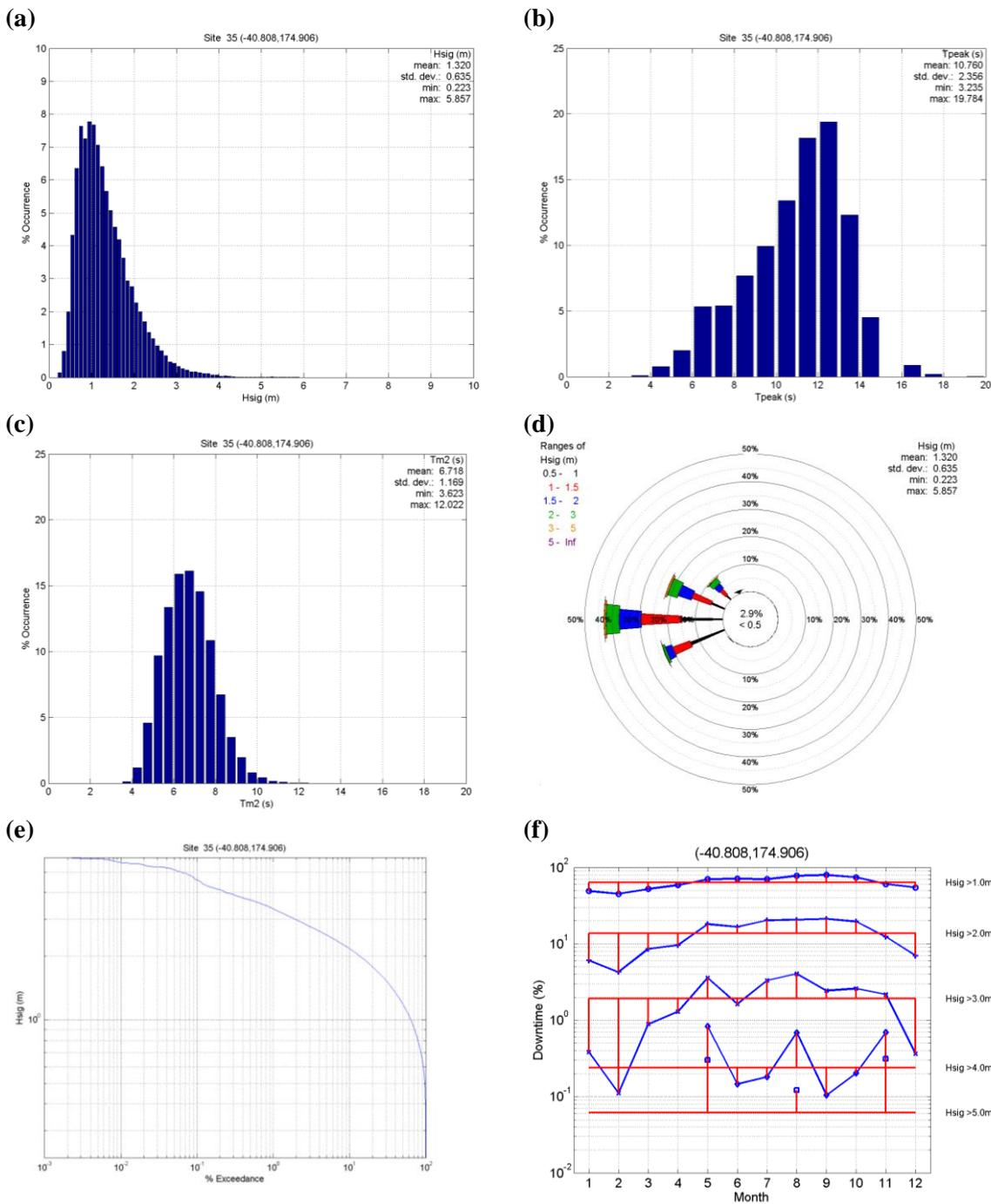
**Figure 2.17. Occurrence statistics for site 35 at (40.808°S, 174.906°E) from the full 1979-1998 hindcast. The first three plots show percentage occurrence for (a) significant wave height, (b) peak wave period, and (c) mean wave period (second moment). Also shown are (d) the wave rose, (e) the wave height exceedance distribution, and (f) “downtime”, i.e. the percentage of time that given significant wave height thresholds are exceeded for each month.**
